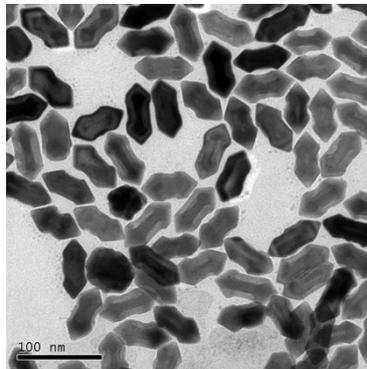
**Figure S4** TEM image of Au730@Au NPs without Cys pre-incubation before overgrowth.
