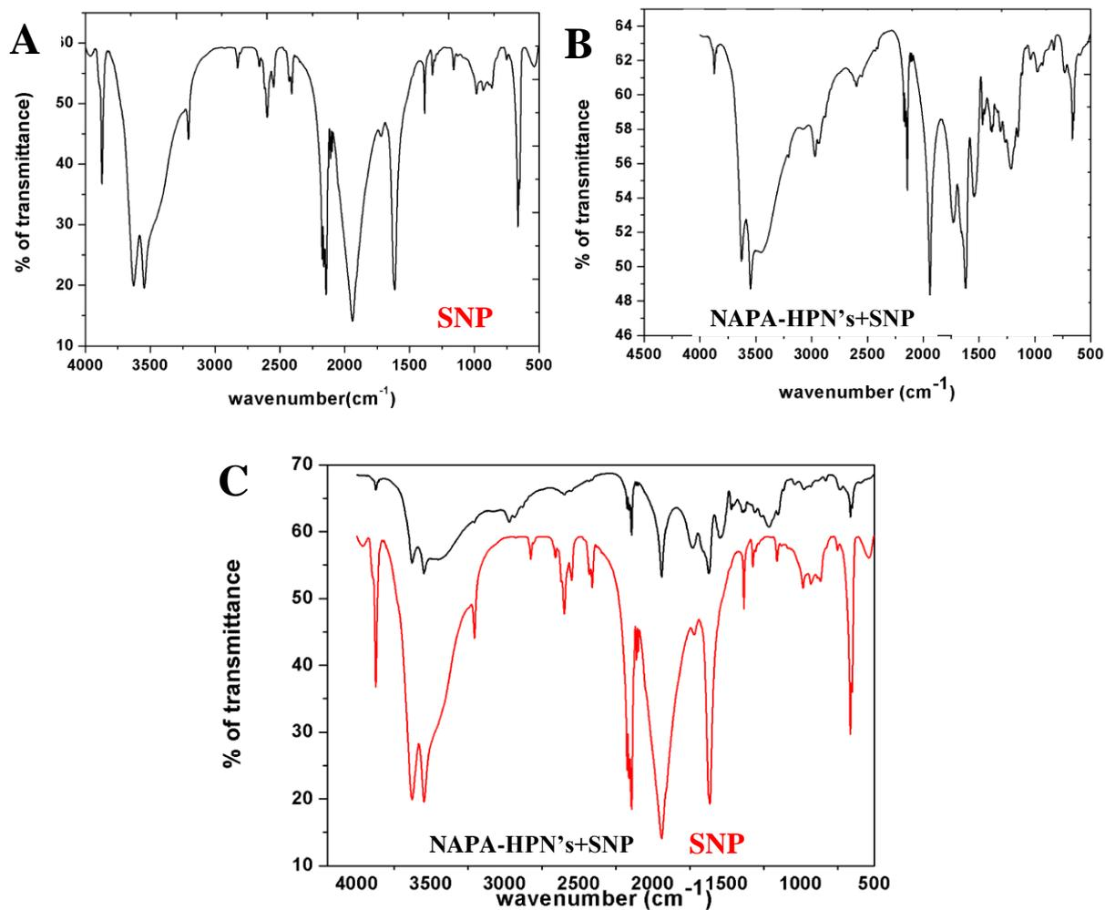
**Figure S7.** FTIR images of (A) SNP. (B) NAPA-HPN's+SNP and (C) overlap of both A and B showing the physical the physical entrapment of SNP by NAPA-HPN's.
