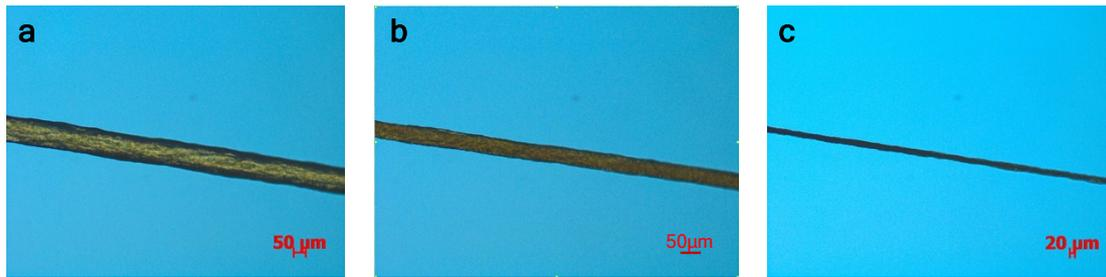
**Figure S2.** The shrink of GO gel fiber from radial direction. The POM images of GO gel fiber after 0s (a), 45s (b) and 90s (c).
