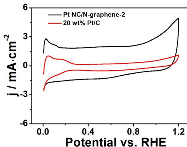
**Figure S6.** CVs of Pt NC/N-graphene-2 and 20 wt% Pt/C in  $N_2$ -saturated 0.5 M  $H_2SO_4$  solution, indicating the electrochemical active surface areas of 91 and 59  $m^2g^{-1}$  for Pt NP/N-graphene-2 and 20 wt% Pt/C catalysts, respectively.
