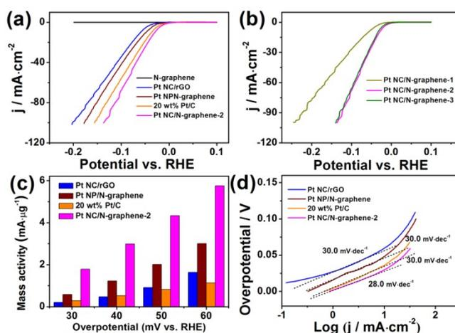
**Figure S4.** (a) LSV curves of N-graphene, Pt NC/rGO, Pt NP/N-graphene, 20 wt% Pt/C and Pt NC/N-graphene-2 catalysts without the iR-compensation; (b) LSV curves of different Pt NC/N-graphene catalysts without the iR-compensation; (c) the mass activity of all catalysts at the different overpotentials; and (d) the corresponding Tafel plots derived from (a).
