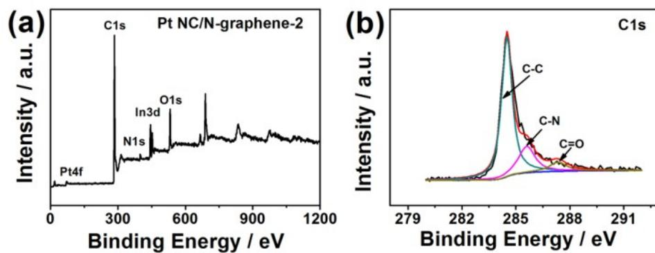
**Figure S2.** The full (a) and high-resolution C1s (b) XPS spectra of Pt NC/N-graphene-2.
