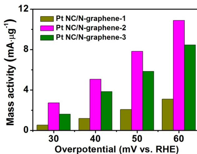
**Figure S5.** The mass activities of Pt NC/N-graphene-1, Pt NC/N-graphene-2 and Pt NC/N-graphene-3 with the iR-compensation.
