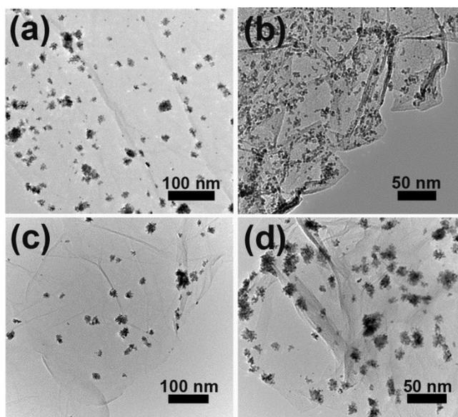
**Figure S3.** TEM images of (a) Pt NC/rGO, (b) Pt NP/N-graphene, (c) Pt NC/N-graphene-1 and (d) Pt NC/N-graphene-3.
