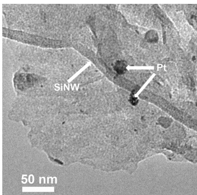
**Figure S1.** TEM image showing Pt was grown between a SiNW and N-graphene.
