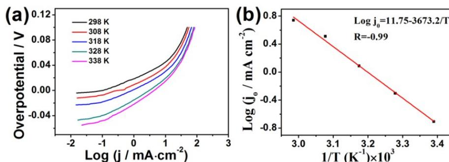
**Figure S7.** (a) Tafel curves of Pt NC/N-graphene-2 at different temperatures without the  $iR$ -compensation; and (b) the corresponding Arrhenius plot.
