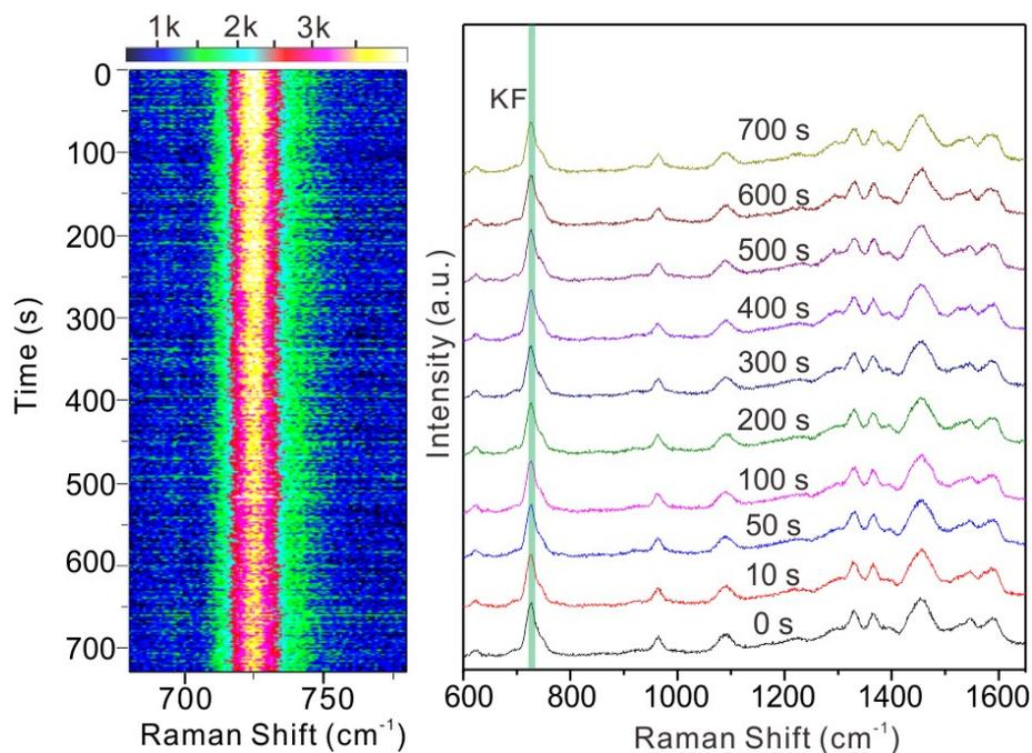
**Fig. S4** (a) the alteration of 2D SERS mapping at 700-780  $\text{cm}^{-1}$  with increasing time.
