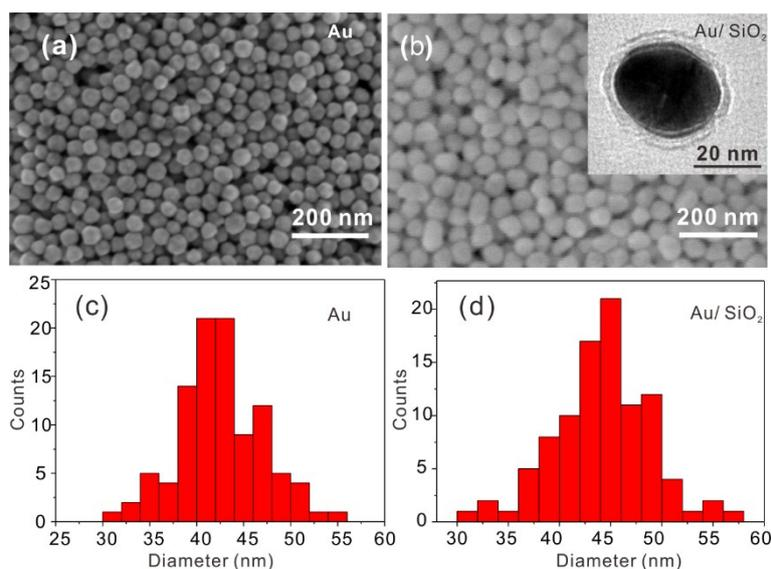
**Fig. S7** The SEM of the different materials. (a) Au NPs (b) Au/SiO<sub>2</sub> The inset shows the TEM of the Au/SiO<sub>2</sub>. The size-distribution histogram of (c) Au nanoparticles and (d) Au/SiO<sub>2</sub>.
