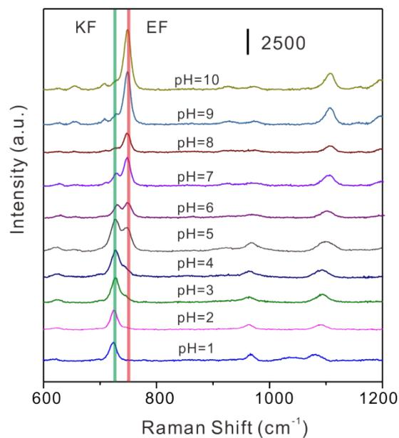
**Fig. S1** SERS spectra of different pH hypoxanthine solution in the presence of Au NPs.
