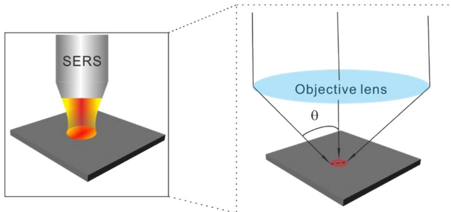
**Fig. S6** The diagram of the Objective lens and spot size.
