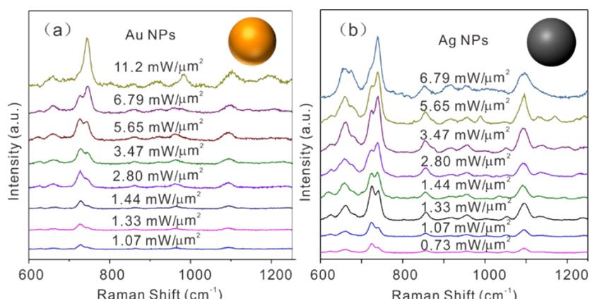
**Fig. S8** Power densities-dependent SERS spectra of Hypoxanthine at different SERS structure. (a) Au NPs (b) Ag NPs The all SERS spectra were collected with 1 s integration time.
