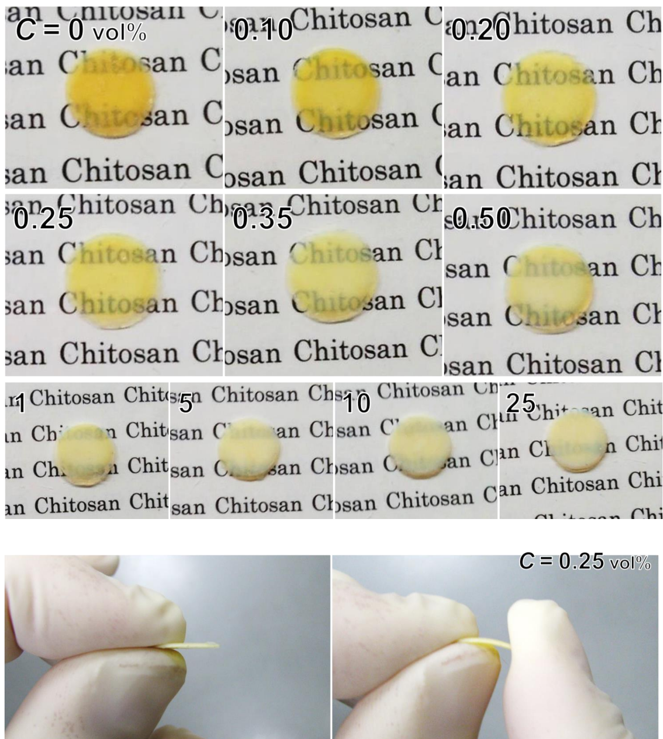
Figure S19. Photographs of the samples after the compression test. The compressed sample bended to some extent by hand (bottom).
