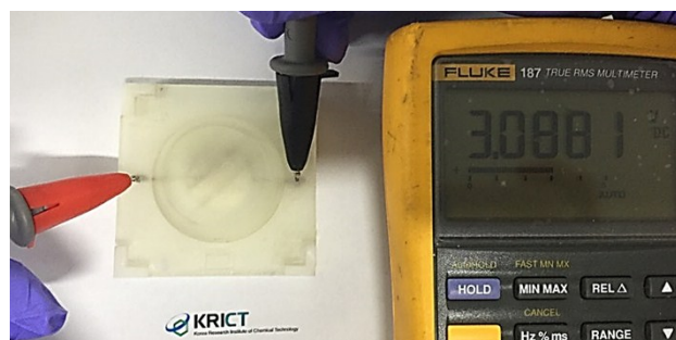
Figure S6. Photograph of a well-formed interconnection between the lower and upper levels showing the voltage output of the battery embedded on the lower level.
