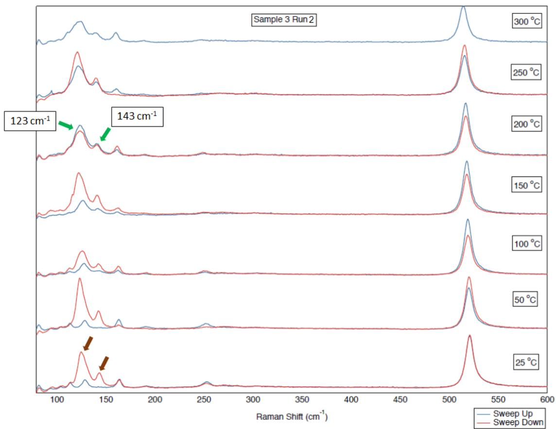
Fig. S6. Raman spectra of encapsulated 1T'-MoTe<sub>2</sub> at various temperatures for Sample 3, Run 2 (Ar flow).
