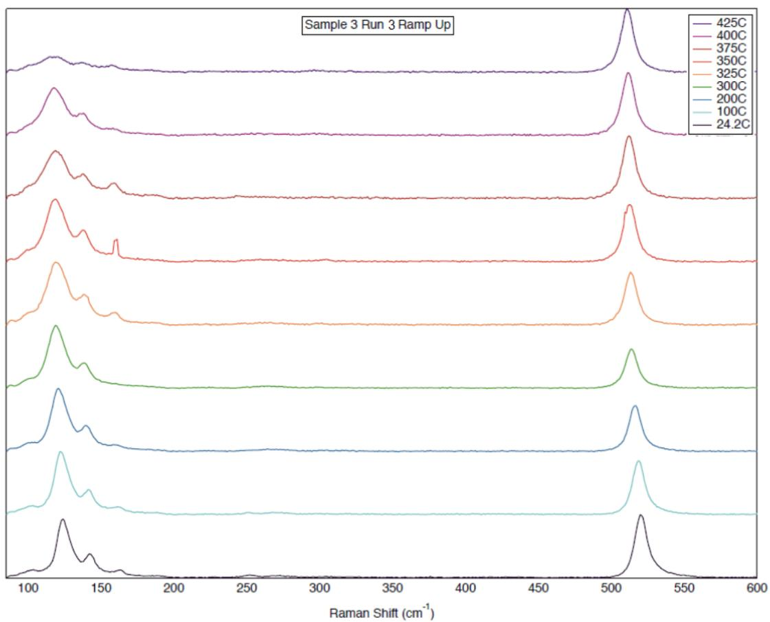
Fig. S7. Raman spectra of encapsulated 1T'-MoTe<sub>2</sub> at various temperatures for Sample 3, Run 3 (Ar flow). No MoTe<sub>2</sub> Raman signal was observed at and above 450 °C.
