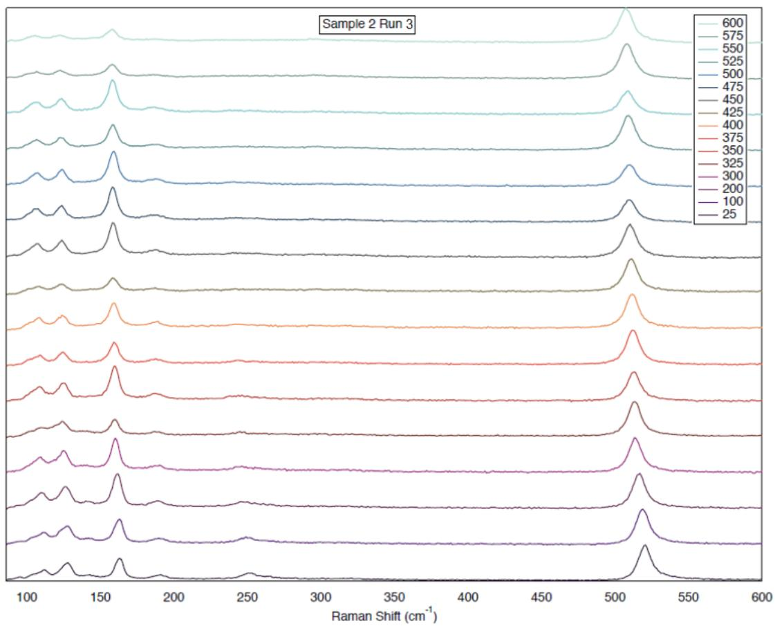
Fig. S5. Raman spectra of encapsulated 1T'-MoTe<sub>2</sub> at various temperatures for Sample 2, Run 3 (Ar flow).
