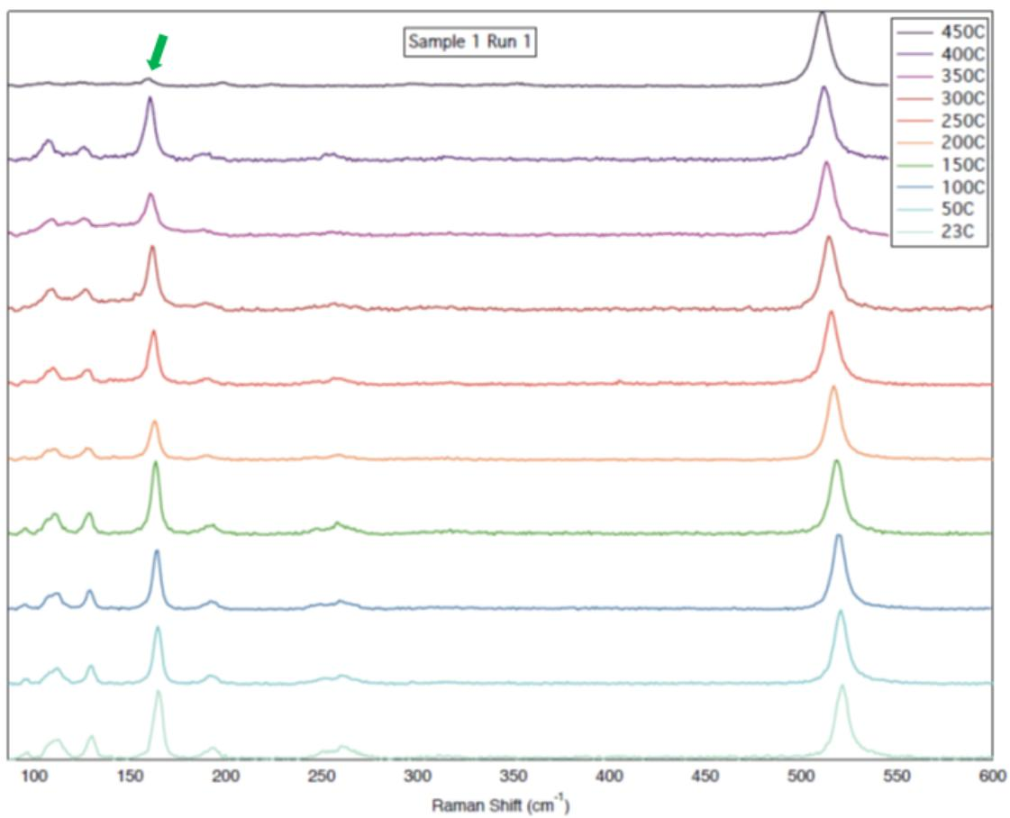
Fig. S2. Raman spectra of encapsulated  $1\text{T}'\text{-MoTe}_2$  at various temperatures for Sample 1, Run 1 (in air). The green arrow points to position of the strongest initial  $\text{MoTe}_2$  peak at room temperature,  $\sim 164 \text{ cm}^{-1}$ .
