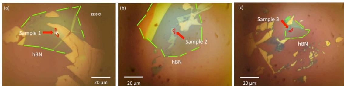
Fig. S1. Optical micrographs of (a) Sample 1, (b) Sample 2, and (c) Sample 3, at room temperature, before heating. Red outlines denoting the thinnest region of the flake, which is probed by Raman scattering, and green outlines denoting the edges of the encapsulating hBN.
