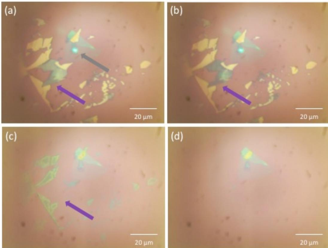
Fig. S4. Optical micrographs of Sample 3, Run 2 at (a) 250 °C, (b) 300 °C, and then after (c) 375 °C and (d) 400 °C, both taken at 100 °C. The gray arrow in (a) indicates where the sample was probed at all temperatures while the purple arrows in (a), (b), and (c) show the decomposition of small, uncovered flakes below and to the left of the sample, which is complete in (d).
