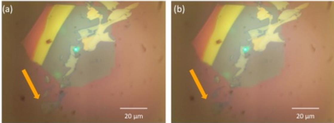
Fig. S3. Optical micrographs of Sample 2 during Run 2 at (a) 250 °C and (b) 300 °C. The orange arrows indicate the decomposition of small, uncovered flakes under and to the left of the sample in this temperature range.
