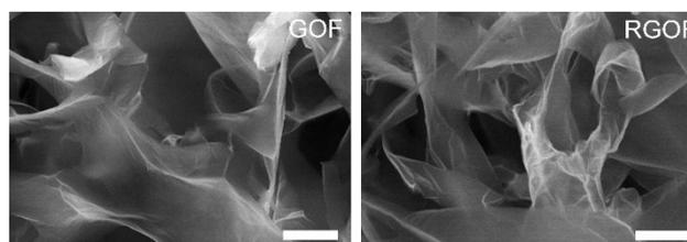
**Fig. S3** SEM images of the GOF (a) and RGOF (b). They separately correspond to the EDX images in Figure 2c and d. The scale bars are 20 μm in panels (a) and (b).
