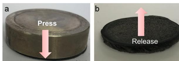
**Fig. S2** The real-time images of the compression–recovery process. Diameters: 4.5 cm.
