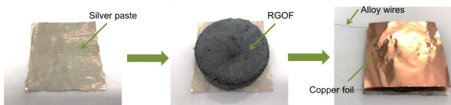
**Fig. S5** Fabrication process of the RGOF-based sensor device.
