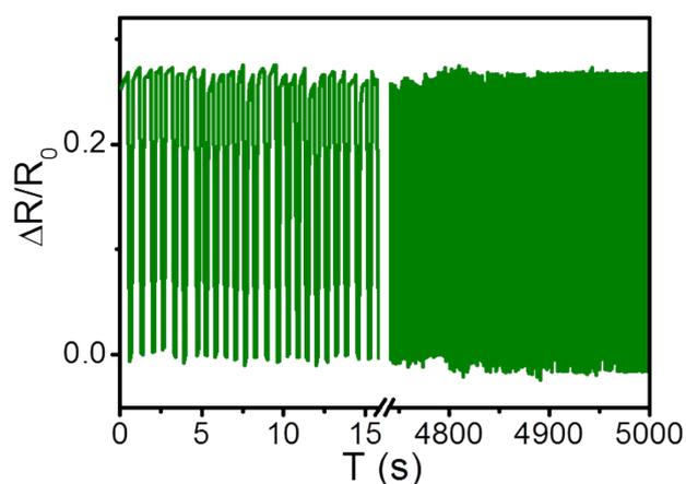
**Fig. S7** The stability test of the RGOF sensor under a pressure of 13 Pa for more than 5000s cycles (in 5000 s).
