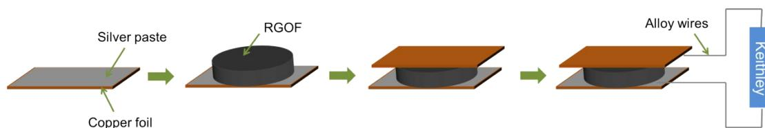
**Fig. S6** Schematic of the fabrication process of the rGO foam-based sensor device.
