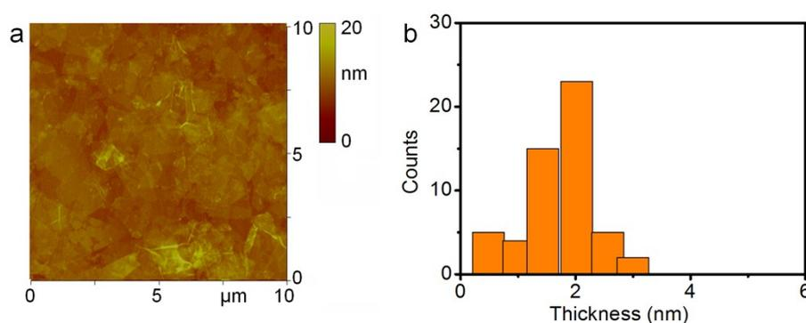
**Fig. S1** AFM image of the GO nanofilms (a) and statistical information of the thickness of the GO sheets (b).
