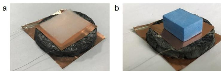
**Fig. S9** The RGOF sensor under a pressure of  $\sim 0.1$  Pa (a) and 13 Pa (b).
