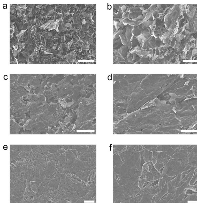
**Fig. S8** a,b) SEM images of the initial RGOF without compression. c,d) SEM images of the compressed RGOF after the long-term cycling pressure test with large pressure (over 300 Pa). e,f) SEM images of the initial RGO sheet without compression. The scale bars in panels (a-f) are 200, 100, 200, 100, 50, and 25  $\mu\text{m}$ .
