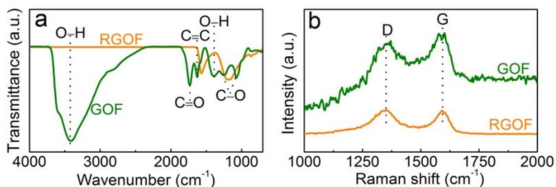
**Fig. S4** a) FTIR spectra of the GOF and RGOF. In contrast to the GOF, the O–H bond in RGOF disappears, and the C–O and C=O bonds also decrease. b) Raman spectra of the GOF and RGOF. The intensity ratios of D and G peaks for the GOF and RGOF are simulated to be 0.94 and 1.02, respectively.
