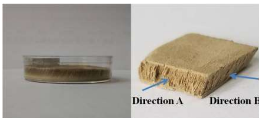
Fig. S3 Digital photographs of hierarchical porous scaffolds.
