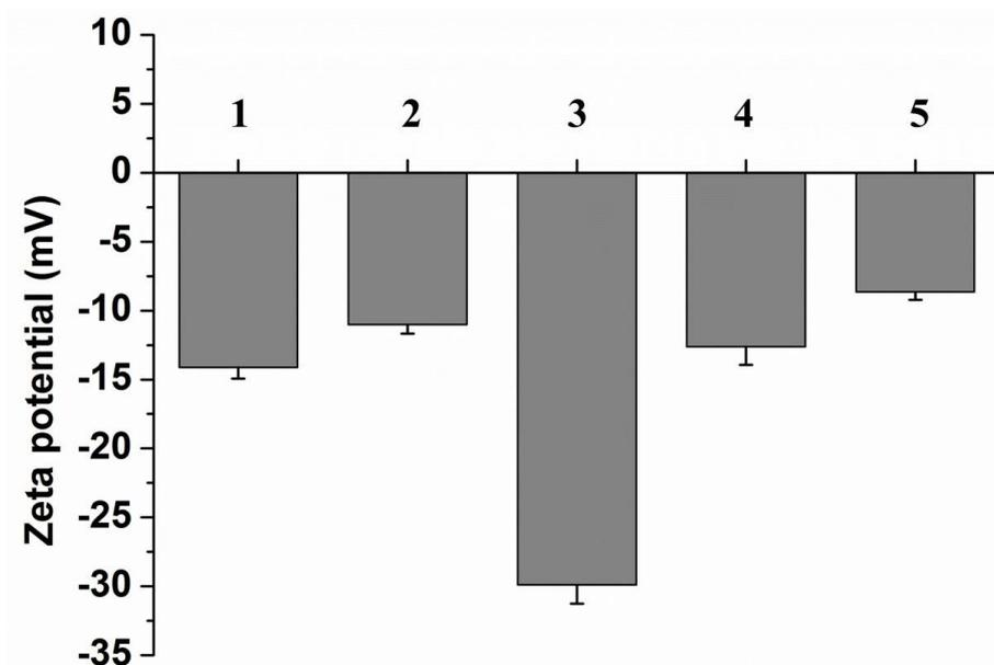
**Figure S5.** Zeta potential of various samples. 1: MSNs, 2: MSNs-CHO, 3: MSNs-siRNA 4: MSNs-siRNA@DOX and 5: MSNs-siRNA@DOX-PEG-FA.
