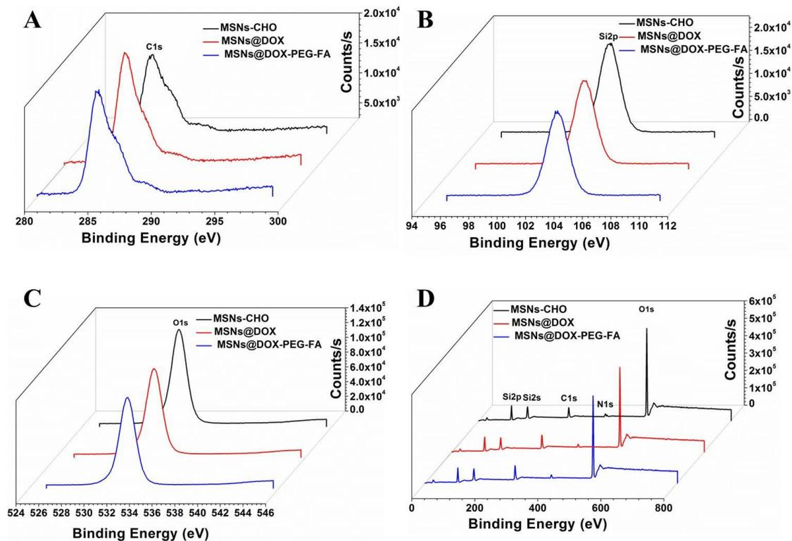
**Figure S6.** XPS spectra of MSNs-CHO, MSNs@DOX, and MSNs@DOX-PEG-FA:
