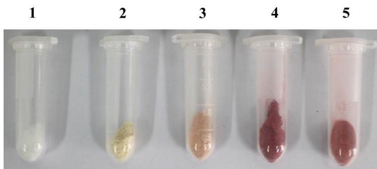
**Figure S1.** Photos of various samples. 1: MSNs, 2: MSNs-CHO, 3: MSNs-DOX (MSNs-CHO:DOX = 1:0.5, m/m), 4: MSNs@DOX (MSNs-CHO:DOX = 1:0.5, m/m), 5: MSNs@DOX-PEG-FA.
