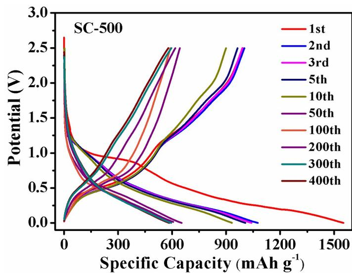
Fig. S3 Charge/discharge voltage profiles of SC-500 composite for the 1 st, 2 nd, 3 rd, 5 th, 10 th, 50 th, 100 th, 200 th, 300 th and 400 th cycles at 200 mA g<sup>-1</sup>.
