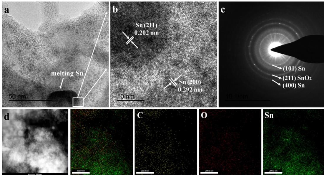
Fig. S5 (a) TEM, (b) high-resolution TEM and (c) SAED pattern of SC-400 electrode after 200 cycles; (d) is the STEM image of the SC-400 composite and the corresponding C, O and Sn EDS elemental mapping.
