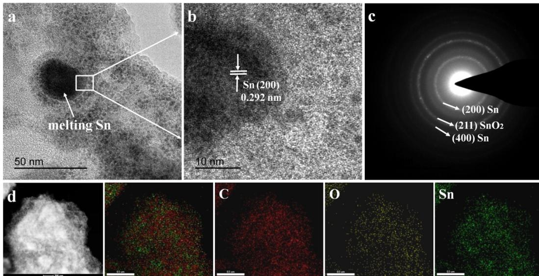
Fig. S6 (a) TEM, (b) high-resolution TEM and (c) SAED pattern of SC-600 electrode after 200 cycles; (d) is the STEM image of the SC-600 composite and the corresponding C, O and Sn EDS elemental mapping.
