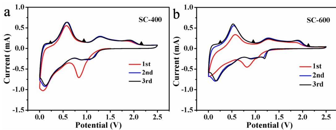
Fig. S4 The cyclic voltammetry curves of (a) SC-400 and (b) SC-600 composite electrodes at  $0.1 \text{ mV s}^{-1}$  in the potential range 0.001-2.5 V.
