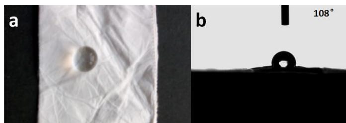
Fig. S14 (a) A photograph of PVDF fibrous membrane. (b) Contact angle of water against of PVDF fibrous membrane after treated with ethyl acetate.
