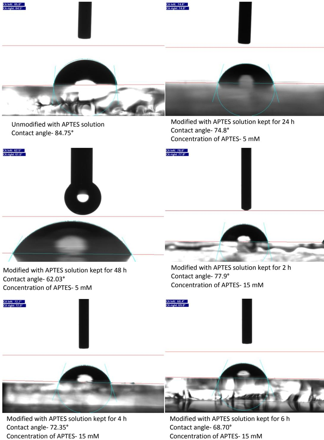
**Figure S5.** Change in contact angle of the samples with 5 mM and 15 mM concentration of APTES solution at different time. The change in contact angle with 5 mM APTES solution is not much effective and the contact angle for 15 mM APTES solution after 24 h was shown in Figure 1(c).
