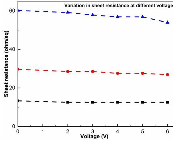
**Figure S12.** Variation in sheet resistance at different voltage for different transparent healable heater based on AgNWs.
