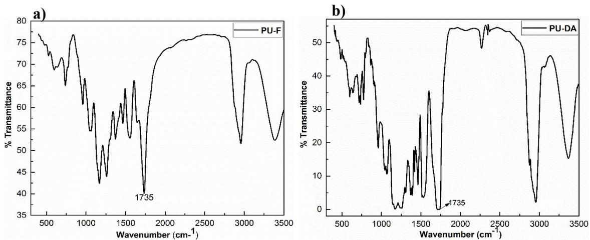
Figure S2. (a) FTIR spectra of polyurethane modified with furyl moiety (PU-F). b) FTIR spectra of PU-DA (Healable polymer). The absorption band at 1735 cm<sup>-1</sup> corresponds to the urethane stretching and indicates that the polymerization was complete.
