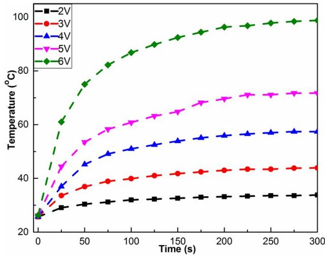
**Figure S13.** Time – dependent temperature profiles at different input voltage with specified sheet resistance of 29.7 Ω /□.
