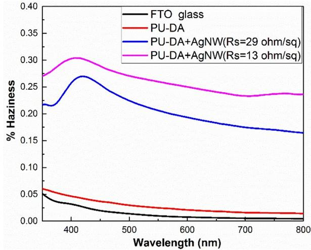
**Figure S8:** Haze factor of the PU-DA polymer with and without silver nanowires.
