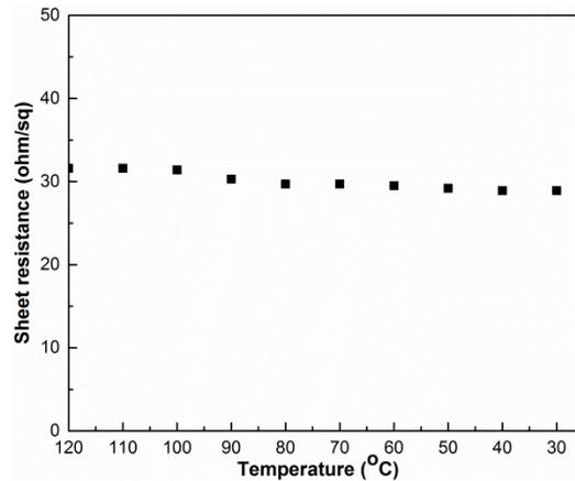
**Figure S11.** Sheet resistance change of a healable heater film with change in temperature. The film heater was cooled from 120 °C to RT and for every decrease in temperature the film was kept for 2 min at that temperature.
