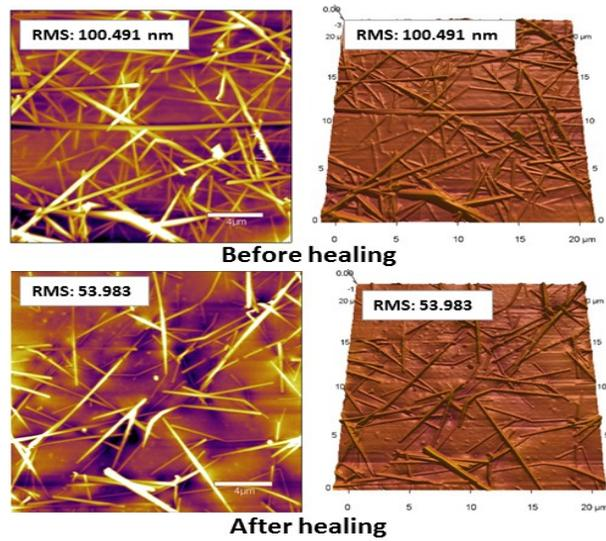
**Figure S10.** Surface roughness of the transparent electrode (TE) before and after healing. The surface roughness of the transparent electrode before and after healing was 100.491 nm and 53.983 nm respectively.
