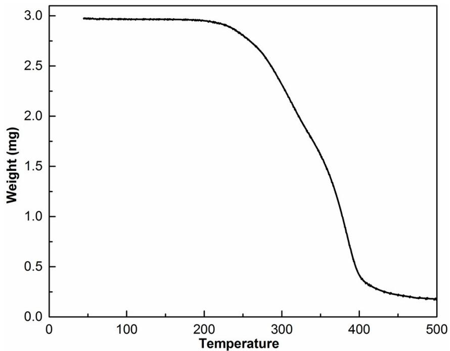
**Figure S4.** TGA curve of the healable polymer. The working temperature of this polymer is below  $220\text{ }^\circ\text{C}$  because the weight loss of the polymer starts from the temperature above  $200\text{ }^\circ\text{C}$ .
