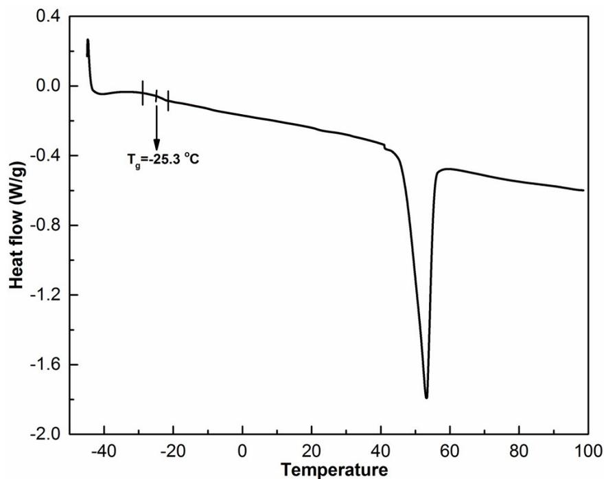
**Figure S3.** DSC of the healable polymer (PU-DA). The glass transition temperature ( $T_g$ ) of the polymer is  $-25.3\text{ }^\circ\text{C}$
