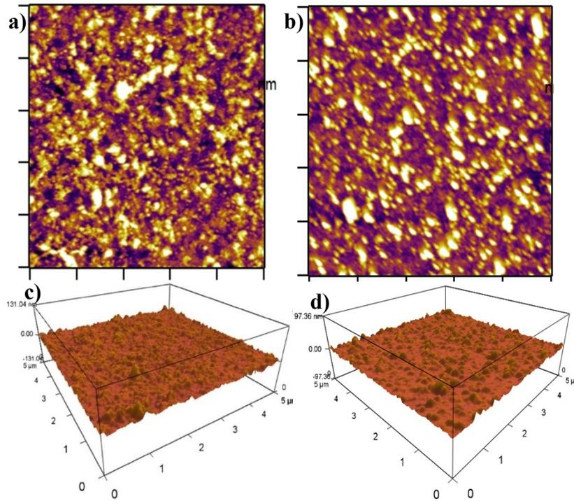
**Figure S7.** AFM images in 2D and 3D with and without APTES treatment. The RMS value of unmodified and modified sample was 4.8 nm and 4.3 nm respectively. (a) & (c) were the images of the sample without APTES treatment and (b) & (d) were the images of the sample with 15 mM APTES treatment.
