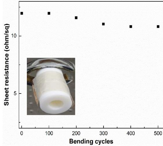
**Figure S9.** Sheet resistance change of the sample with the number of bending and unbending cycle/times. The image inset in the bending-unbending graph shows the sample was wrapped around a 20 mm diameter cylinder
