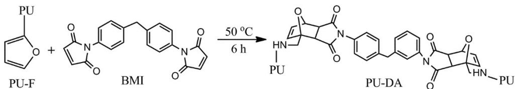
Figure S1. The detailed chemical scheme for the synthesis of PU-DA (Healable polymer)
