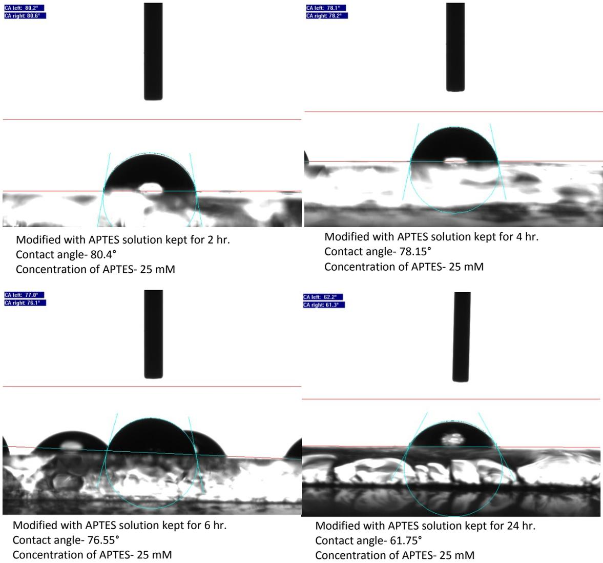
**Figure S6.** Change in contact angle of the samples with 25 mM concentration of APTES solution at different time
