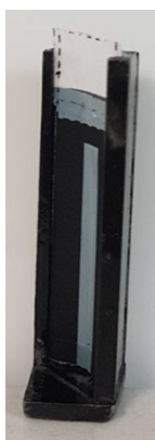
Fig. S1: (a) The creation of test zones with hydrophobic barrier (black areas) and with desired patterns (multiwall and two-dimensional cuvette patterns) through direct-printing a toner layer onto the dried BC nanopaper films using an office laser printer. (b) The fabricated sample holder for recording fluorescence spectra of the developed NRFSA platforms
