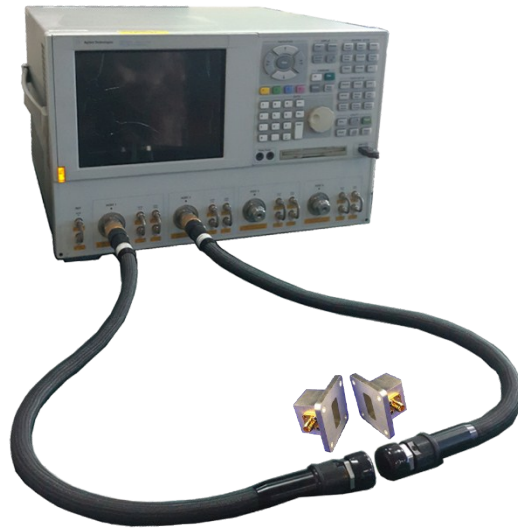
Fig. S3 The experiment setup (Vector network analyzer and waveguide sample holder) for EMI shielding measurement (S-parameters).
