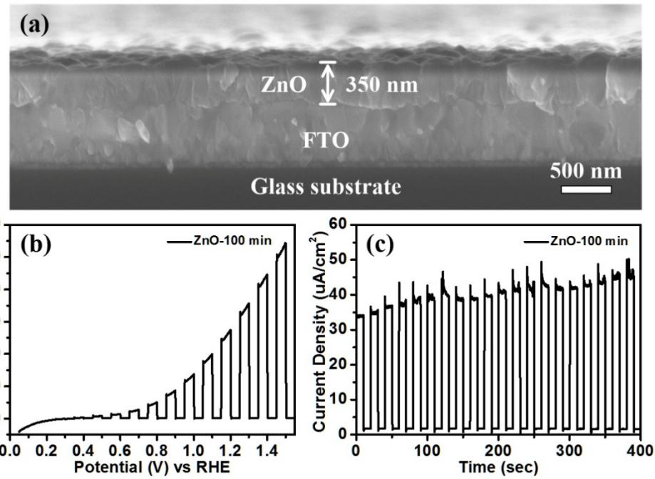
**Fig. S7** (a) Cross-sectional SEM image, (b) LSV curve and (c) Amperometric I-t curve at 1.23 V vs. RHE under chopped AM 1.5G simulated solar illumination for the ZnO thin film with the deposition time of 100 min.
