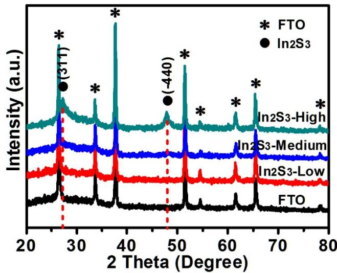
**Fig. S3** XRD patterns of  $\text{In}_2\text{S}_3$  NSAs prepared with varied  $\text{In}^{3+}$  concentrations.
