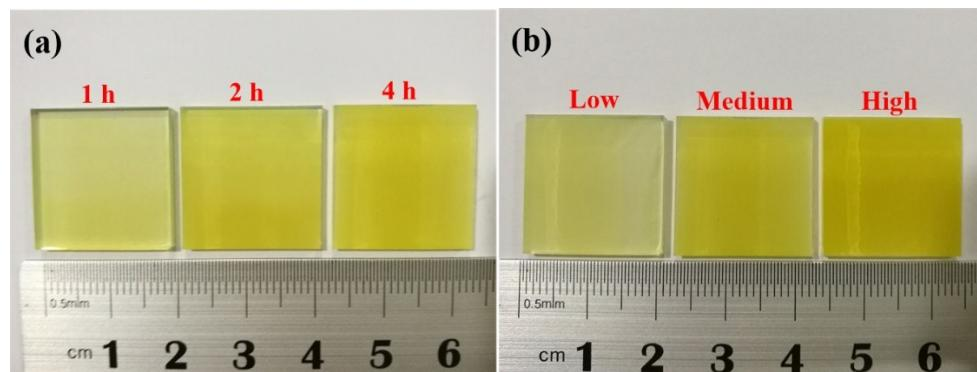
**Fig. S1** Optical images of  $\text{In}_2\text{S}_3$  NSAs grown on FTO substrates with (a) different reaction times and (b)  $\text{In}^{3+}$  concentrations.
