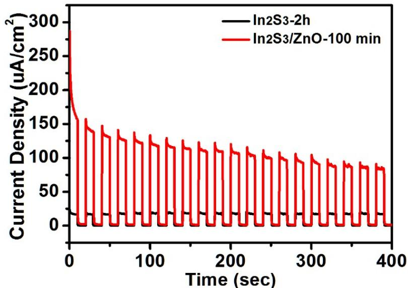
**Fig. S11** Amperometric I-t curves of the  $\text{In}_2\text{S}_3$ -2h and  $\text{In}_2\text{S}_3/\text{ZnO}$ -100 min NSAs at 1.23 V vs. RHE under chopped AM 1.5G simulated solar illumination.
