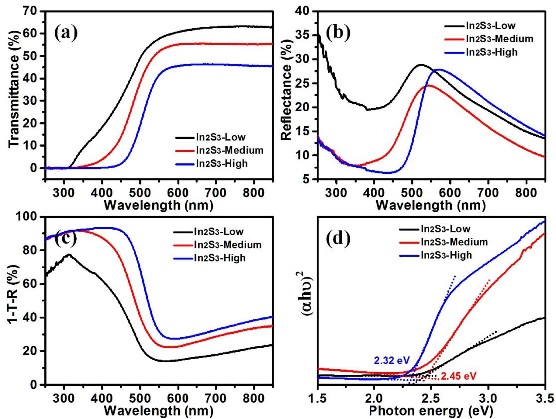
**Fig. S4** (a) Transmission spectra, (b) reflection spectra, (c) absorption spectra and (d) energy bandgap determination of the  $\text{In}_2\text{S}_3$  NSAs prepared with varied  $\text{In}^{3+}$  concentrations.
