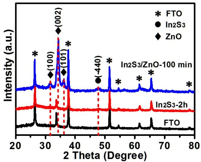
**Fig. S5** XRD patterns of FTO substrate, pristine  $\text{In}_2\text{S}_3$ -2h NSAs and  $\text{In}_2\text{S}_3$ /ZnO-100 min NSAs.
