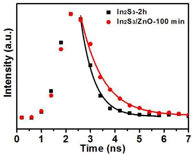
**Fig. S10** Time-resolved PL spectra of the In<sub>2</sub>S<sub>3</sub>-2h and In<sub>2</sub>S<sub>3</sub>/ZnO-100 min NSAs.
