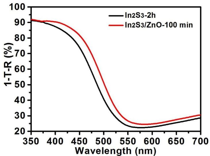
**Fig. S9** Absorption spectra of the In<sub>2</sub>S<sub>3</sub>-2h and In<sub>2</sub>S<sub>3</sub>/ZnO-100 min NSAs.
