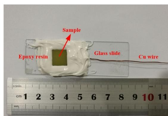
**Fig. S2** Optical image of a home-made photoanode based on  $\text{In}_2\text{S}_3$  NSAs.
