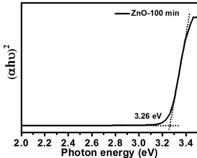
**Fig. S6** Energy bandgap determination of the ZnO film grown on FTO substrate with the sputtering time of 100 min (thickness: 350 nm).
