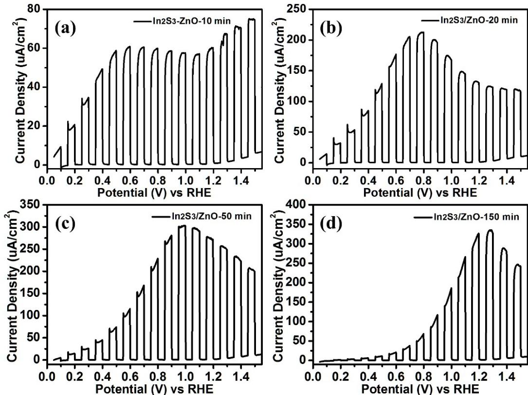
**Fig. S8** LSV curves of the  $\text{In}_2\text{S}_3/\text{ZnO}-x \text{ min}$  NSAs at 1.23 V vs. RHE under chopped AM 1.5G simulated solar illumination: (a-d) 10, 20, 50 and 150 min, respectively.
