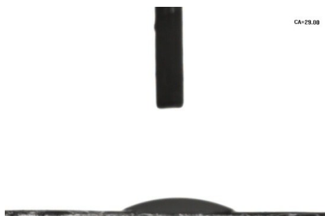
Figure S2. Optical images showing contact angles (CAs) of ink drops on the surface of nitrocellulose varnish film
