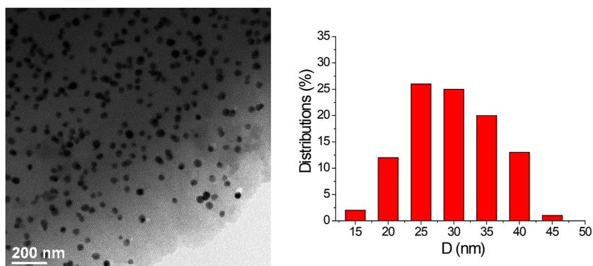
**Fig. S10.** TEM images and the corresponding particle size distributions of the nickel nanoparticles of Ni/OMC-0.1 with stirring time (3h).
