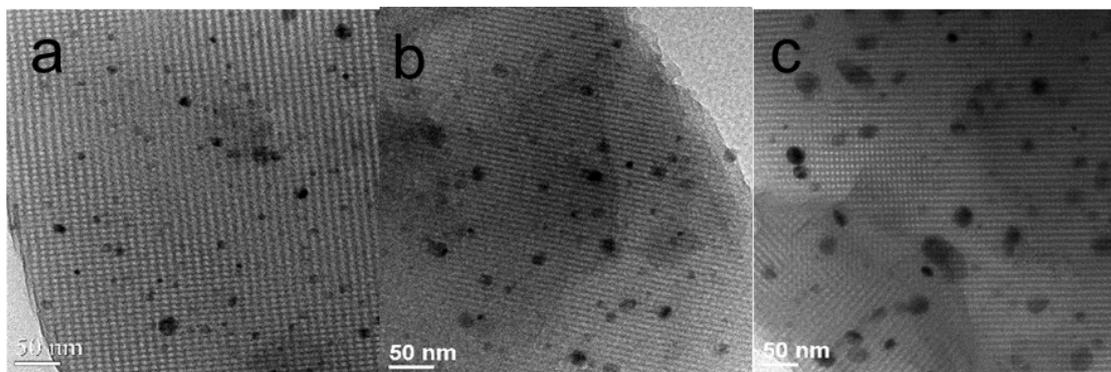
**Fig. S4.** Magnified TEM images of the Ni nanoparticle/OMC composites: (a) Ni/OMC-0.05, (b) Ni/OMC-0.075 and (c) Ni/OMC-0.1.
