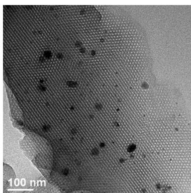
**Fig. S6.** TEM images of Ni/OMC-0.1 after using 7 times.
