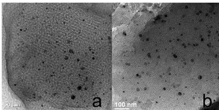
**Fig. S7.** TEM images of Ni/OMC-0.1 with different carbonization temperature: (a) Ni/OMC-0.1 carbonized at 600°C and (b) Ni/OMC-0.1 carbonized at 750°C.
