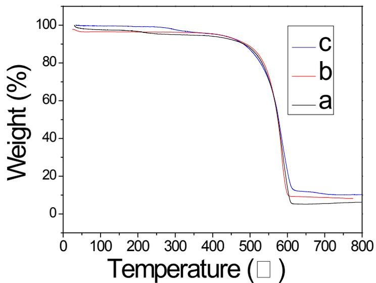
**Fig. S2.** TGA curves of the Ni nanoparticles/OMC composites with different Ni contents: (a) Ni/OMC-0.05, (b) Ni/OMC-0.075, (c) Ni/OMC-0.1.
