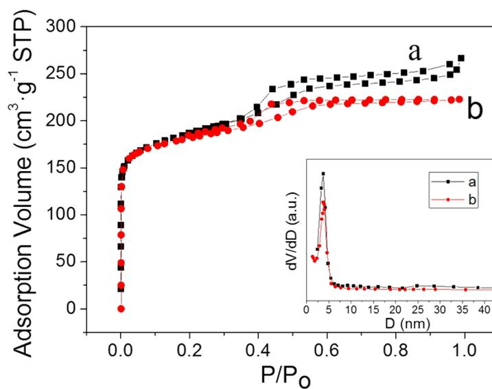
**Fig. S8.** N<sub>2</sub> sorption/desorption isotherms and the corresponding pore size distribution curve (inset) of OMC/Ni-0.1 with different carbonization temperature: (a) Ni/OMC-0.1 carbonized at 600°C, (b) Ni/OMC-0.1 carbonized at 750°C.
