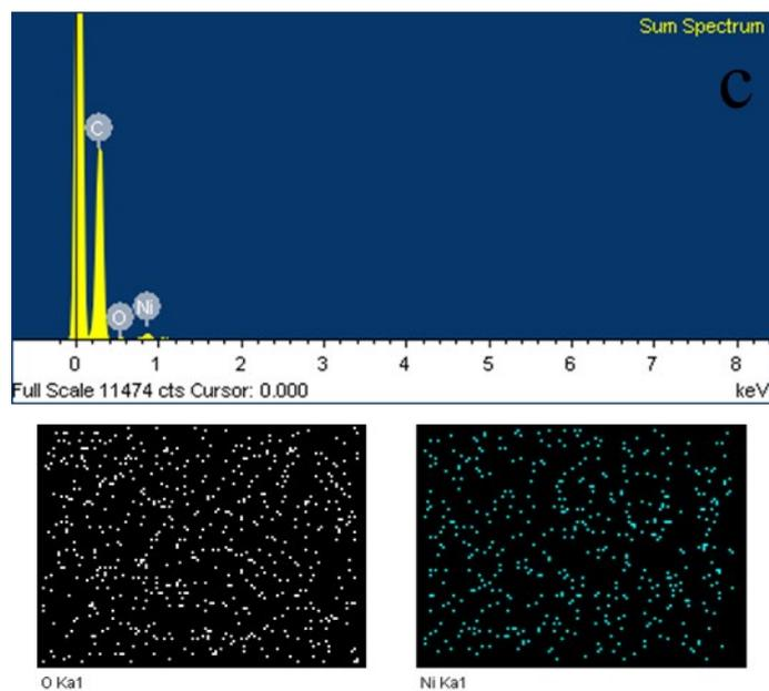
**Fig. S5.** EDX-Mapping images of the Ni nanoparticle/OMC composites: (a) Ni/OMC-0.05, (b) Ni/OMC-0.075 and (c) Ni/OMC-0.1.
