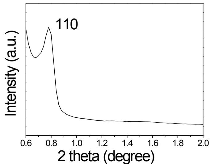
**Fig. S1.** Small-angle XRD pattern of the ordered mesoporous carbon FDU-16.
