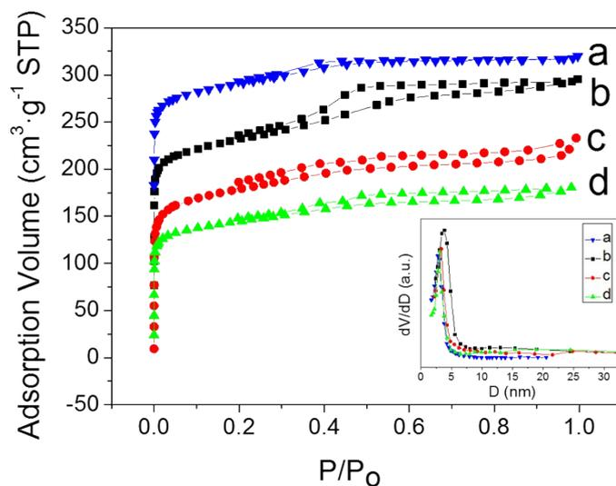
**Fig. S3.** N<sub>2</sub> sorption/desorption isotherms and the corresponding pore size distribution curve (inset) of the Ni nanoparticles/OMC composites with different Ni contents: (a) FDU-16, (b) Ni/OMC-0.05, (c) Ni/OMC-0.075, (d) Ni/OMC-0.1.
