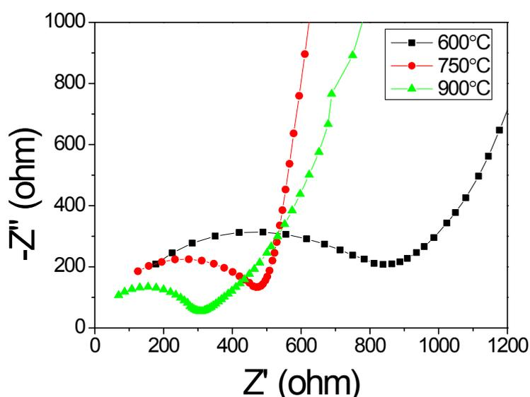
**Fig. S9.** Nyquist plots of electrochemical impedance spectroscopy (EIS) for Ni/OMC-0.1 with different carbonization temperature.
