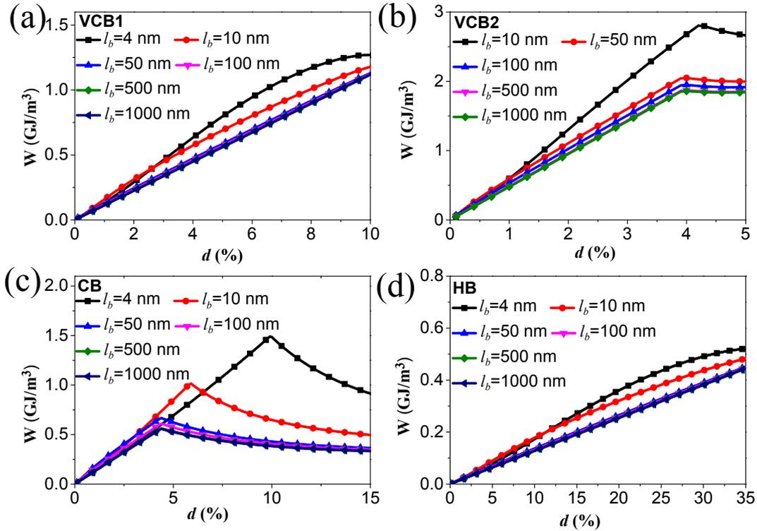
**Fig. S2** Plots of the calculated effective toughness of graphene-based artificial nacres with brittle interface as a function of the crosslink density under different sizes of the graphene sheets for (a) VCB1, (b) VCB2, (c) CB and (d) HB crosslinks.
