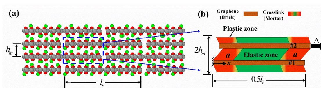
**Fig. S1** (a) Schematics of the brick (graphene)-and-mortar (crosslinks) structure and representative volume element (RVE, as highlighted as the dash box); (b) Schematics of a nonlinear shear-lag model with elastic-perfectly-plastic interface under tension (plastic zone, as highlighted as the red zone; elastic zone, as highlighted as the green zone).
