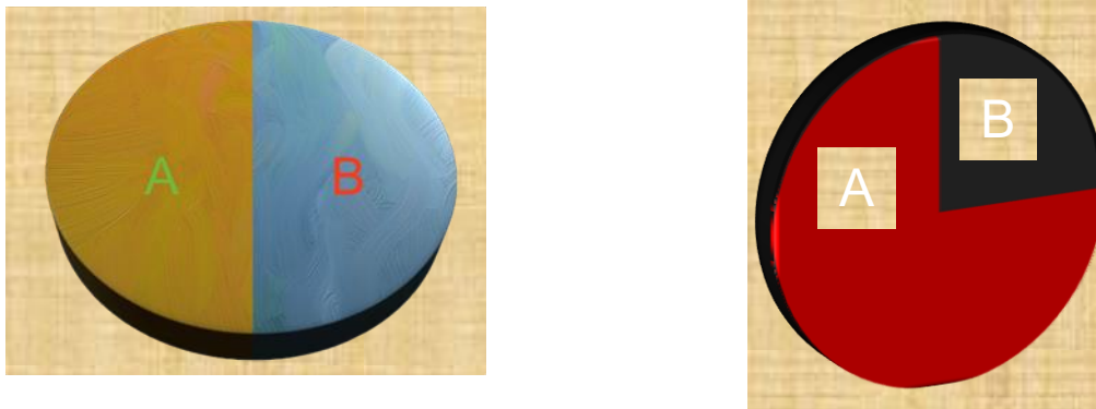
Figure S6. Showing different types of section target arrangement used for the production of nanoparticles.
