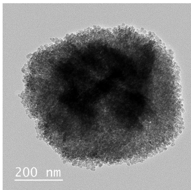
**Fig. S1** TEM image of FeCaP<sub>30</sub> samples. Note that the FeCaP microspheres are made of dense agglomeration of the primary nanoparticles.
