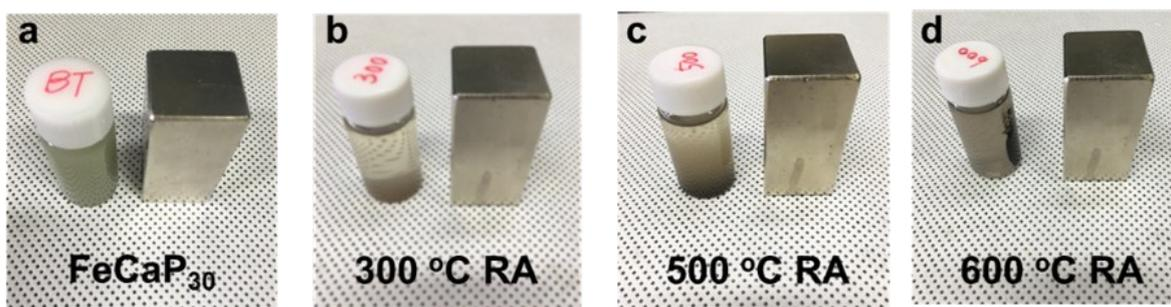
**Figure S5.** Fe/FeCaP microspheres dispersed in water exhibited magnetic property on a permanent Nd magnet.
