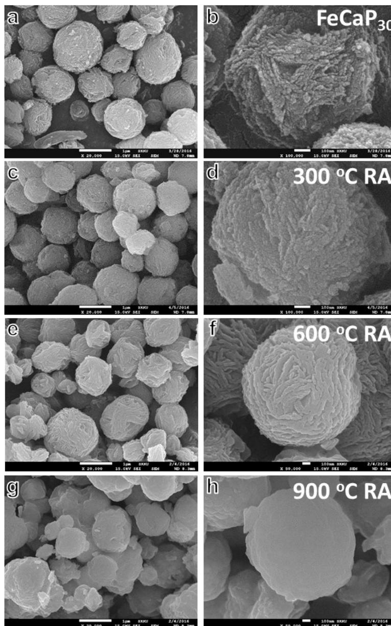
**Fig. S3** Low- and high-magnification SEM images of reduction-annealed FeCaP samples (Before treatment (a, b), 300 °C (c, d), 600 °C (e, f) and 900 °C (g, h)) as a function of annealing temperature.
