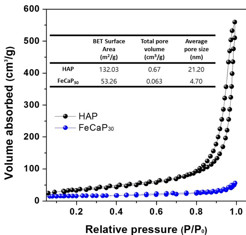
**Fig. S2** N<sub>2</sub> adsorption–desorption isotherms of the synthetic samples of FeCaP<sub>0</sub>(HAP) and FeCaP<sub>30</sub> and the BET surface area, total volume and average pore size of samples are summarized in inset table.
