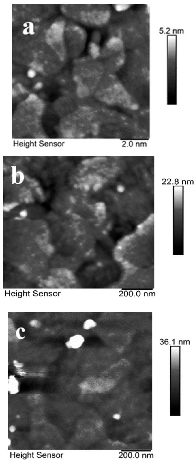
**Fig.S3** AFM image of AuNPs/rGO/AuNPs-10 (a), AuNPs/rGO/AuNPs-30 (b), and AuNPs/rGO/AuNPs-50 (c).
