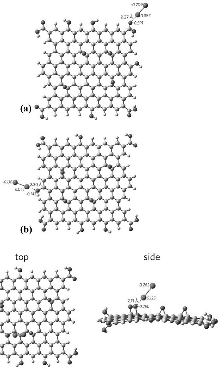
**Fig.S5** Ground state structures of  $\text{Au}_2/\text{rGO}$  complexes optimized at the B3LYP/6-31G//LANL2DZ level at different coordination sites: (a) the carboxylic acid group ( $-\text{COOH}$ ), (b) the hydroxyl group ( $-\text{OH}$ ) and (c) the epoxy groups ( $-\text{O}-$ ). NPA charges (a.u.) for selected atoms are displayed in italics, and bond lengths in  $\text{\AA}$ .
