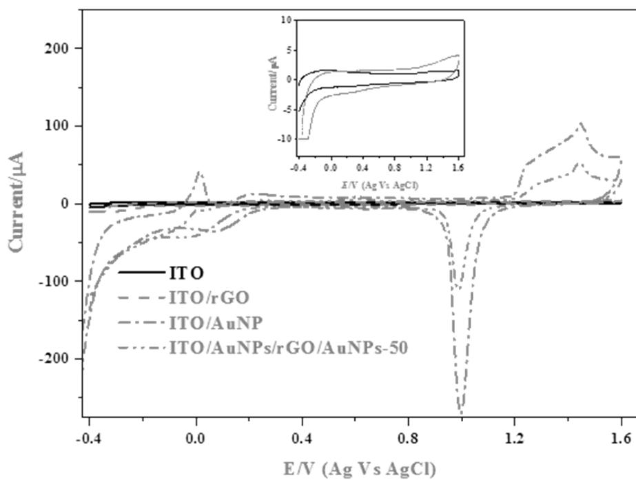
**Fig. S2** CVs of bare ITO (a), ITO/rGO (b), ITO/AuNPs (c) and ITO/AuNPs/rGO/AuNPs-50 (d) in the  $0.5\text{M H}_2\text{SO}_4$  at scan rates  $50\text{mVs}^{-1}$ .
