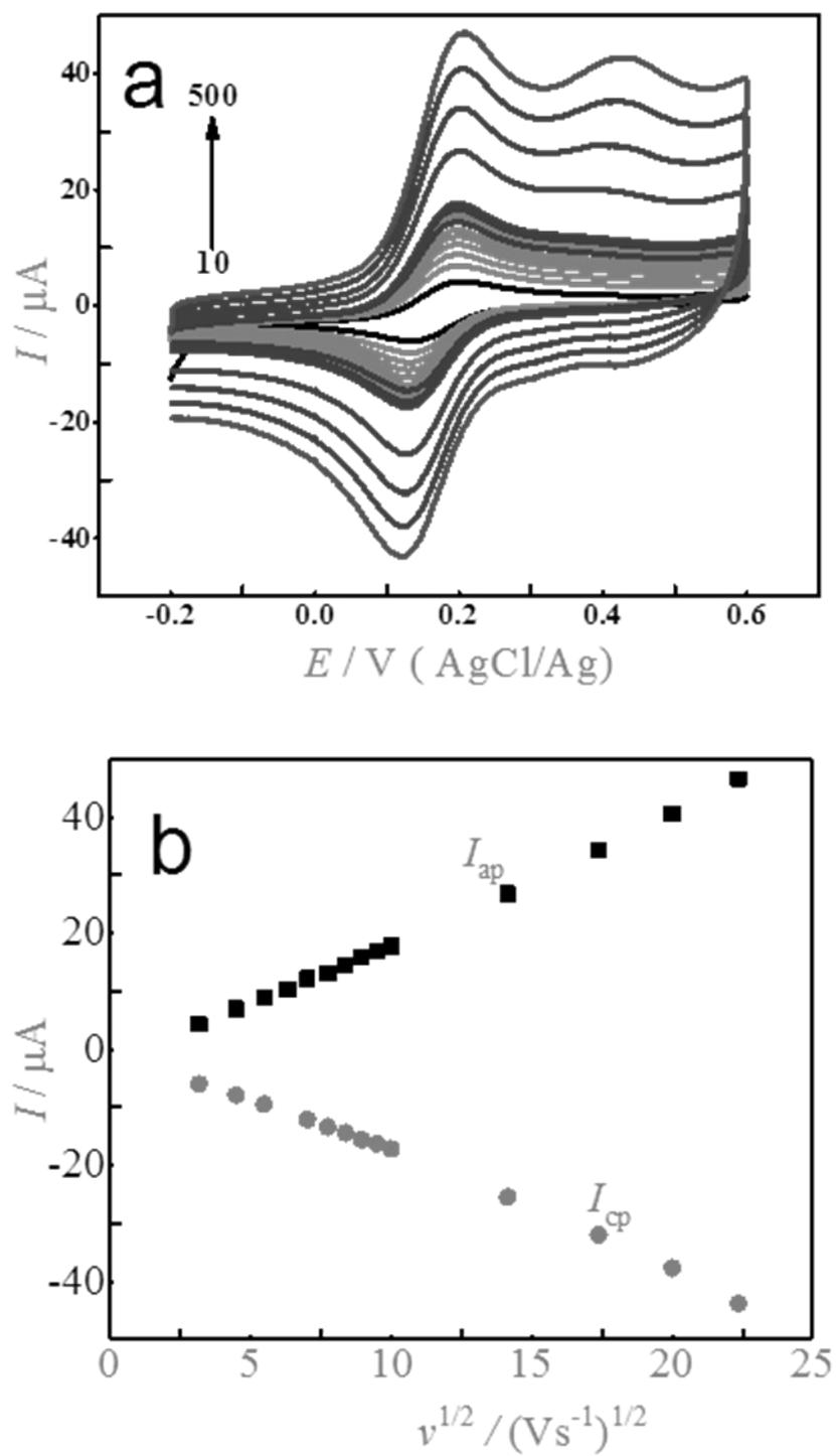
**Fig.S4** CVs of GCE/AuNPs/rGO-50 recorded in PBS at different scan rates of 10, 20, 30, 40, 50, 60, 70, 80, 90, 100, 200, 300, 400, and 500 mVs<sup>-1</sup> in presence of 1mM [Fe(CN)<sub>6</sub>]<sup>3-/4-</sup> (a) and the plot of the  $I$  vs.  $v^{1/2}$  (b)
