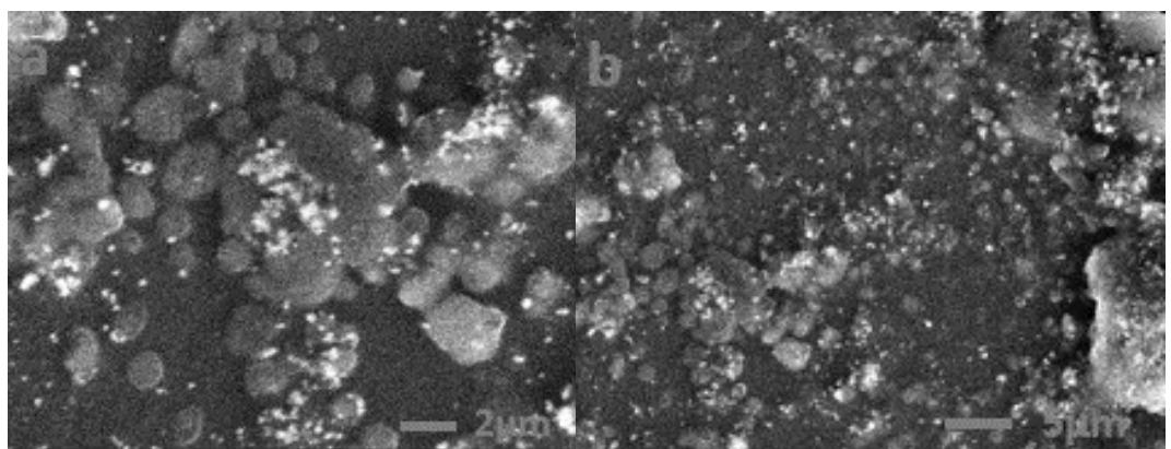
**Fig.S1** SEM images of new method (a, AuNPs/rGO /AuNPs-50) and traditional method (b, rGO-AuNPs-50).
