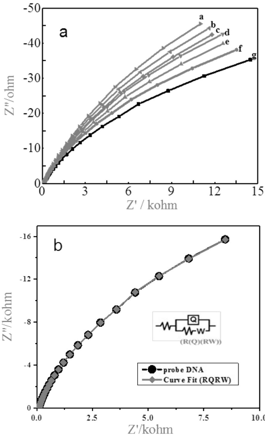
**Fig. S7** (a) Impedance behaviors of probe I on the various cDNA concentrations of (a) 1  $\mu\text{M}$ , (b) 0.1  $\mu\text{M}$ , (c) 0.01  $\mu\text{M}$ , (d) 1 nM, (e) 0.1 nM, (f) 0.01 nM and (g) 1 pM. (b) Nyquist curve fit diagrams of probe (I) was recorded at PBS 10 (pH 7.4) containing 0.1M KCl of 1mM  $[\text{Fe}(\text{CN})_6]^{3-/4-}$  and inset: equivalent circuit fit diagram. Applied DC potential of 250 mV and the AC amplitude of  $\pm 5$  mV.
