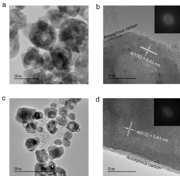
**Fig. S2** (a) TEM image of the NTP/C-6h nanocomposite. It manifests the presence of the holes, which are located in the interior of the particles without channels throughout the whole particles. (b) HRTEM image of the NTP/C-6h nanocomposite. The (110) crystal plane in hexagonal NTP and the coated carbon layer are confirmed. The inset is the SAED pattern. (c) TEM image of the NTP/C-48h nanocomposite. The holes also locate in the interior. (d) HRTEM image of the
