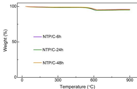
**Fig. S1** TGA curves of the NTP/C nanocomposites performed in air condition. The carbon contents of all the NTP/C nanocomposites are at the same level of  $\sim 5$  wt%.
