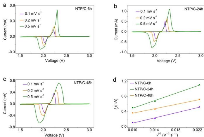
**Fig. S3** (a-c) CV curves of the NTP/C-6h, NTP/C-24h, and NTP/C-48h electrodes at various scan rates, respectively. (d) Linear fittings of the peak current as a function of the square root of the scan rate.
