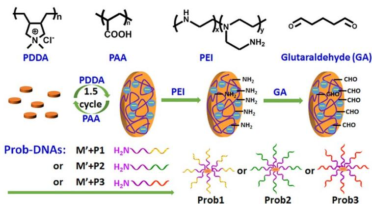
**Scheme S2.** Surface modification process of SU-8 photoresist building blocks.
