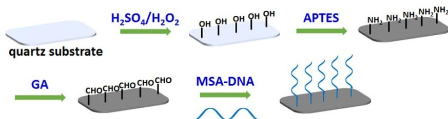
**Scheme S3.** Surface modification process of the substrate for MSA.
