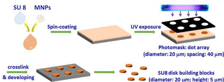
**Scheme S1.** The fabrication process of SU-8 photoresist building blocks.
