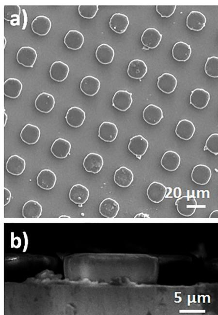
**Figure S1.** SEM images of the as-prepared SU-8 photoresist building blocks
