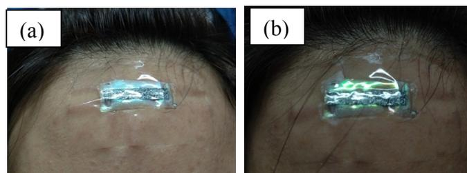
Fig. S10 Photographs of the rGO/IOAC sensor attached on the forehead to monitor sweat during running. (a) the initial sensor; (b) the sensor absorbed sweat after running for about 15 min .
