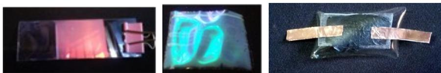
Fig. S3 (a) SiO<sub>2</sub> colloidal crystal template; (b) inverse opal AC film; (c) rGO film fixed on the AC film without microstructure as flexible strain sensor (rGO/AC).
