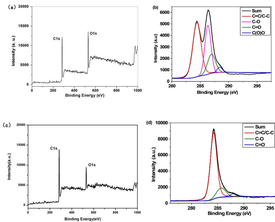
Fig. S2 XPS spectra of GO film (a) and rGO film (c). C1s region of GO film (b) and rGO film (d).
