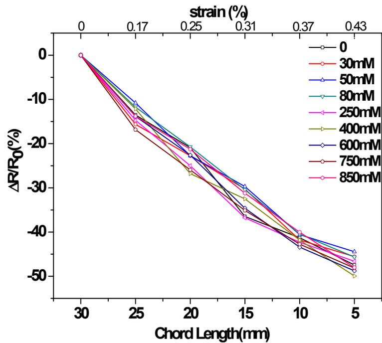
Fig. S9 The bending strain response of the rGO/IOAC sensor while the IOAC substrate absorbed different concentration of NaCl.
