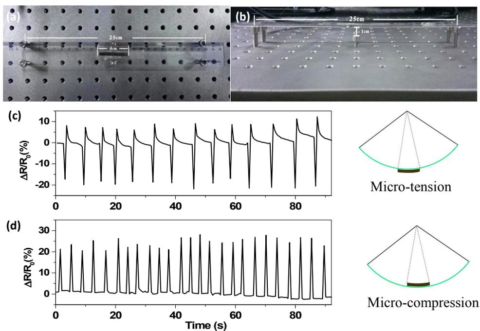
Fig. S5 (a-b) photographs of rGO/IOAC sensor fixed to a flexible surface to detect microstrain structural variation. (d-e) Relative resistance changes of the sensor under the tensile (up) and compressive (down) strain. Right pictures are the monitoring models of the tensile (up) and compressive (down) strain.
