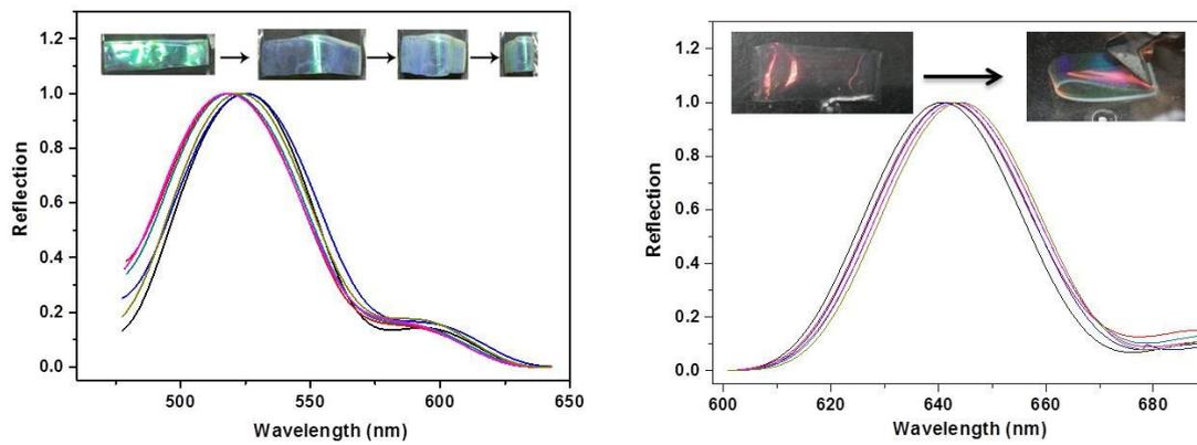
Fig. S8 The structure color and diffraction-peak of the IOAC substrate (left) and the IOAC substrate in artificial sweat (right) under different bending-stretching conditions
