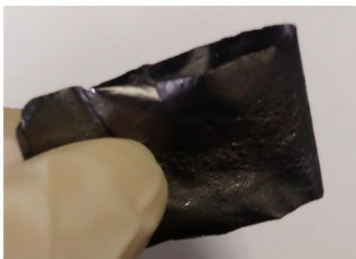
Fig. S1 Photograph of a free-standing rGO film.
