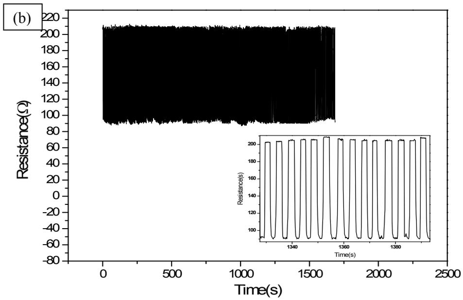
Fig. S6 The resistance values of the rGO/IOAC sensor measured under the multiple bending and relaxed state. (a) 0.17% strain; (b) 0.43% strain; The inset is the magnification
