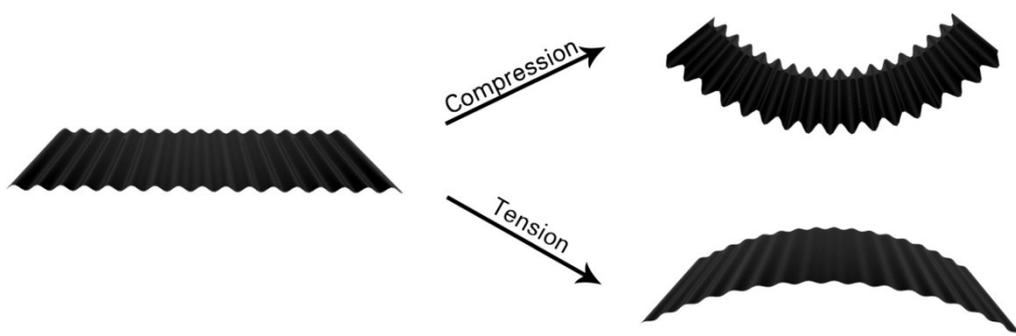
Fig. S4 Schematic illustration of the sensing mechanism.
