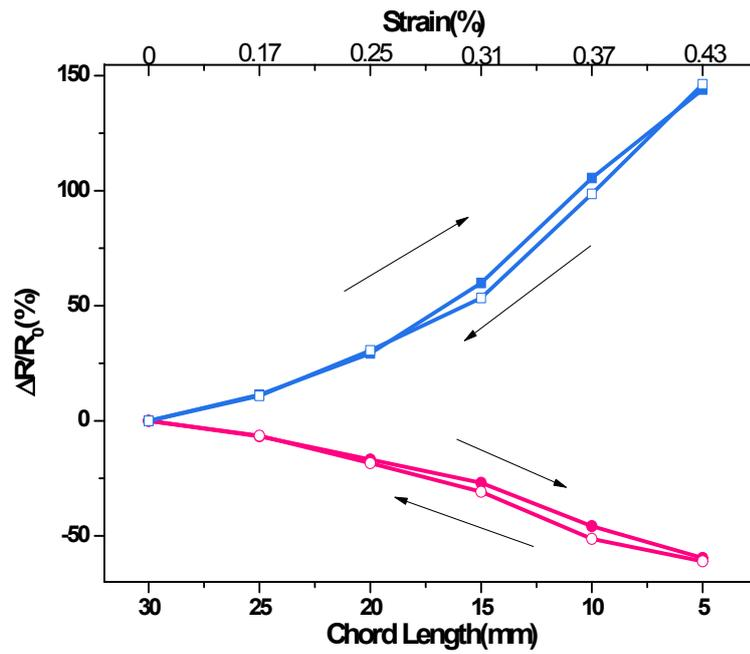
Fig. S7 Resistance change of the rGO/IOAC sensor during strain increase and decrease.
