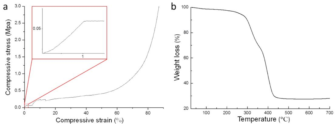
**Figure S7** (a) mechanical resistance and (b) thermal gravimetric analysis of a porous material.
