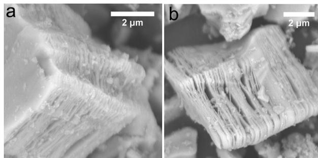
**Figure S1.** SEM images of as-prepared Ti<sub>3</sub>C<sub>2</sub>-MXene.
