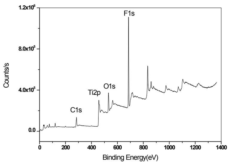
**Figure S2.** XPS spectrum of as-prepared Ti<sub>3</sub>C<sub>2</sub>-MXene.
