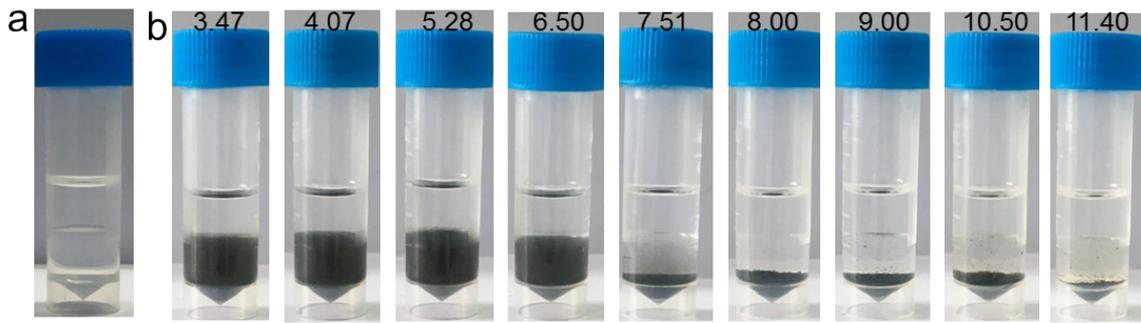
**Figure S4.** The photograph showing (a) the mixture of 1.5ml water, 1.5ml dodecane and CTAB (0.045mM). (b) the mixture of 1.5ml water, 1.5ml dodecane and unmodified  $Ti_3C_2$ -MXene at different pH volume (the MXene concentration=5mg/ml).
