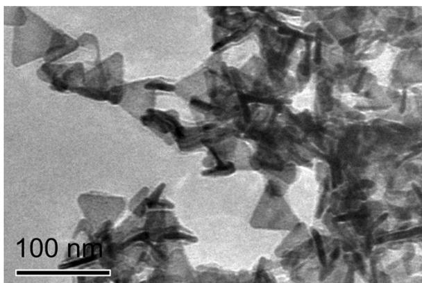
**Fig. S3** TEM image of Au/Ag nanoplates assembling upright on Cu grids, which
