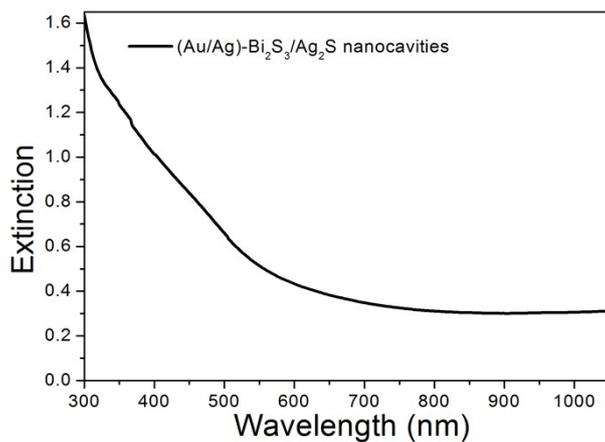
**Fig. S4** The extinction spectrum of (Au/Ag)-Bi<sub>2</sub>S<sub>3</sub>/Ag<sub>2</sub>S hybrid nanocavities.
