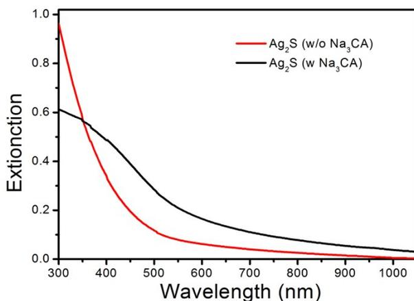
**Fig. S2** The extinction spectra of Ag<sub>2</sub>S nanoparticles prepared with and without adding Na<sub>3</sub>CA.
