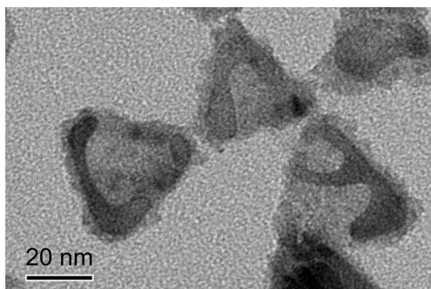
**Fig. S1** TEM image of destroyed nanostructures after CdS nanoparticles were deposited on the Au/Ag nanoplates instead of (Au/Ag)-Ag nanocavities.
