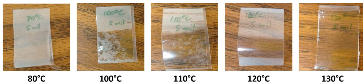
SI Figure 1: Determining minimum viable lamination temperature for EVA/PET film. Temperatures from 80-130°C were tested at a roller force of 50 N and a lamination speed of 2 mm/s
