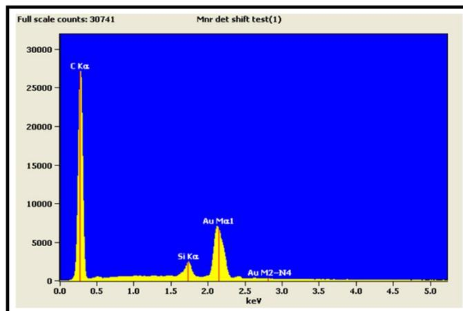
**Figure S4.** Elemental analysis of *mIG*-Au nanobelts. Only the elements of carbon, silicon and gold are recorded in the element spectrum. Note silicon signal originates from the substrate.
