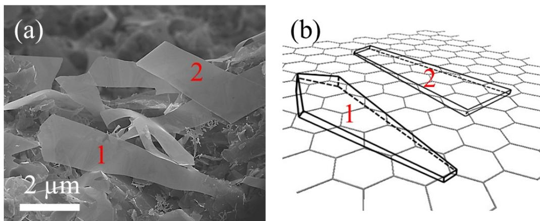
**Figure S7.** (a) Au nanobelts with two representative shapes. (b) Schematic image of two typical Au nanobelts: triangular and straight end.
