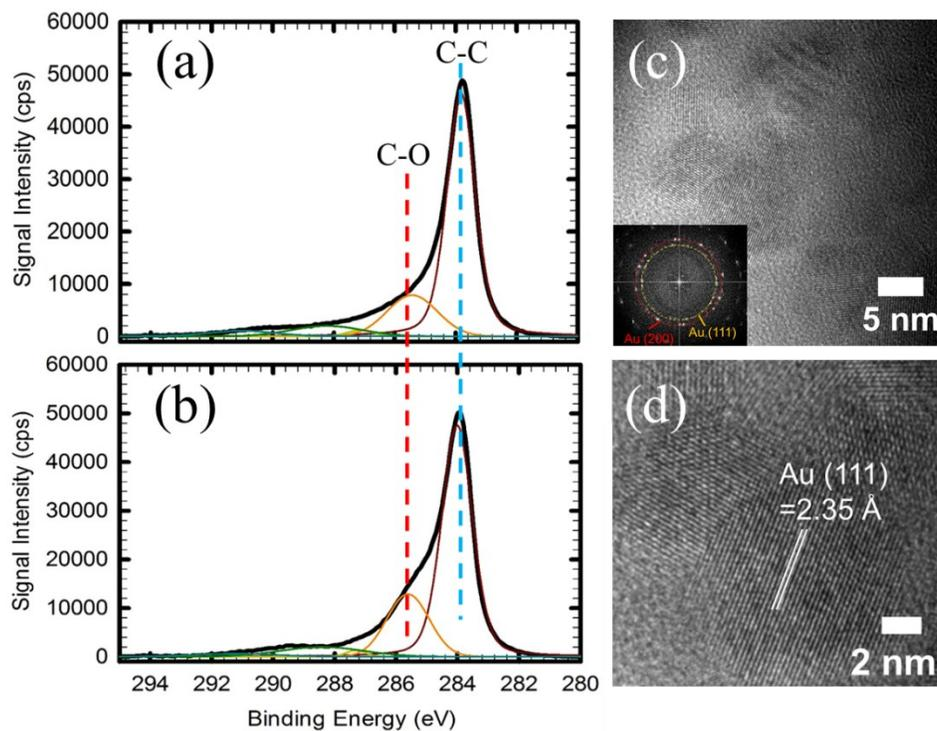
**Figure S9.** Quantification analysis of hydrophilic functional groups on *m*/G before (a) and after (b) oxygen plasma treatment (30 scans) using X-ray photoelectron spectroscopy. (c) A selected area of Au clusters nucleated on plasma oxidized *m*/G (30 scans) at 1 hr and ambient temperature. Inset is the corresponding FFT of the entire area. (d) Atomic structure of Au clusters selected in (c).
