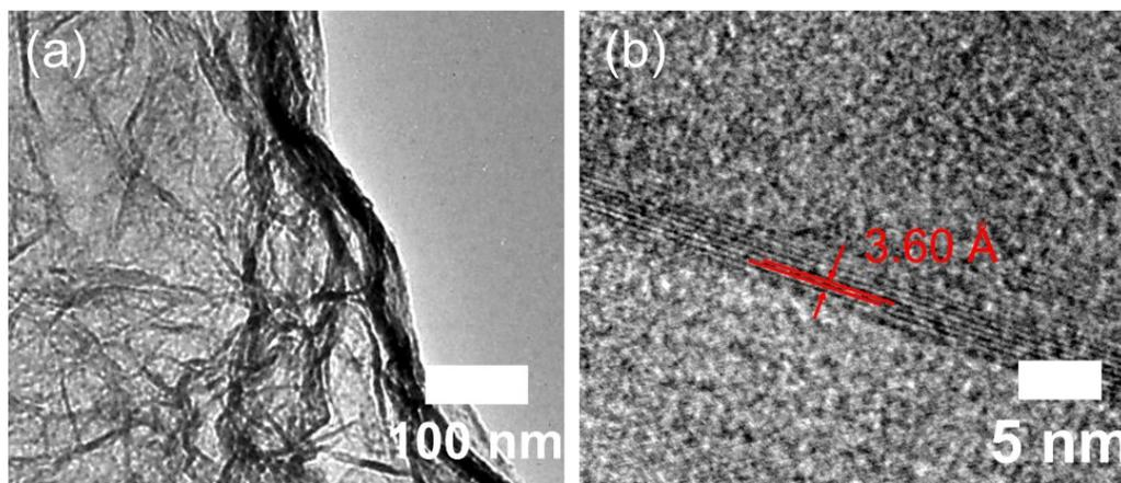
**Figure S1.** (a) Representative TEM image of *m/G* used in this work. (b) High resolution TEM image showing 11-layered graphene edge with the interspace of 3.60 Å.
