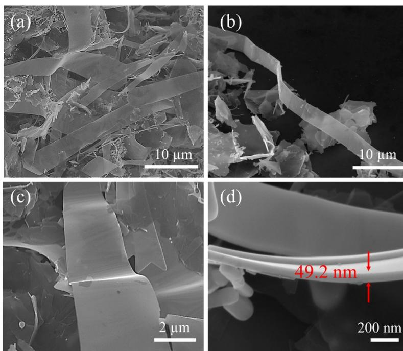
**Figure S3.** Morphologies of *m/G*-Au nanobelts. (a) Au nanobelts lying flat and parallel to the surface of multilayer graphene sheet. (b) An ultralong Au nanobelt isolated from the *m/G* template. (c) Au nanobelts fluctuating on graphene template. (d) Thickness of the nanobelts found to be sub-100 nm.
