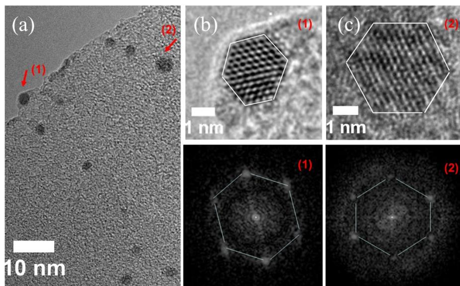
**Figure S5.** (a) TEM image of gold precursor reacting with graphene for 1hr. (b) and (c) Atomic structures and corresponding FFT patterns of two Au nanoplatelets in (a).
