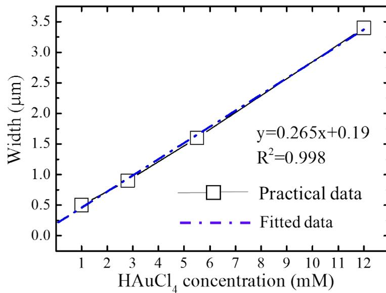
**Figure S10.** The relation between width of Au nanobelts and gold precursor concentrations.
