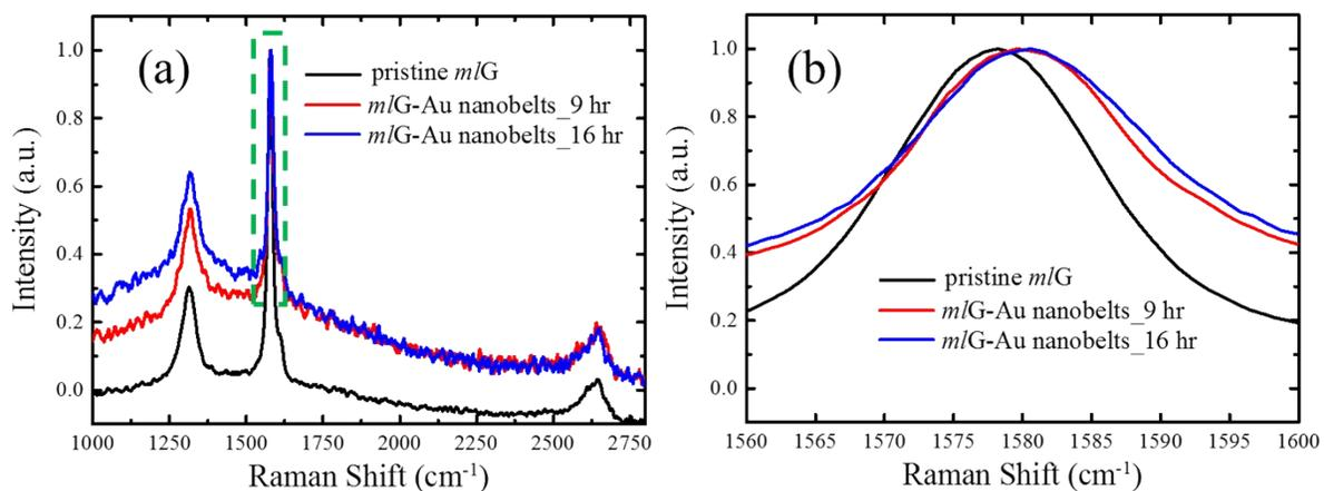
**Figure S2** Raman spectroscopic characterization of *m*/G before and after reaction with gold precursor. (a) Normalized Raman spectra of pristine *m*/G, *m*/G-Au nanobelts at 9 hr and *m*/G-Au nanobelts at 16 hr in the range of 1000  $\text{cm}^{-1}$  to 2800  $\text{cm}^{-1}$ . (b) Raman spectra from 1560  $\text{cm}^{-1}$  to 1600  $\text{cm}^{-1}$  (the green dotted box in (a)) showing slight redshift of G peak with the reaction time.
