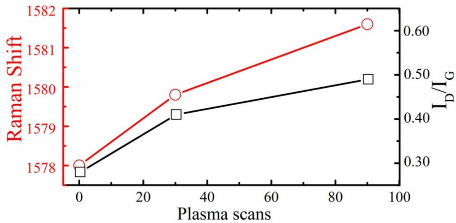
**Figure S8.** Raman shift of G peak and the modification of  $I_D/I_G$  of *m*/G with the number of plasma scans.
