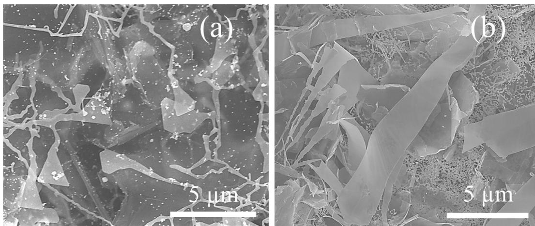
**Figure S11.** Au nanobelts synthesized on *m/G* by using 12.0 mM  $\text{HAuCl}_4$  at the time of (a) 4 hr and (b) 16 hr.
