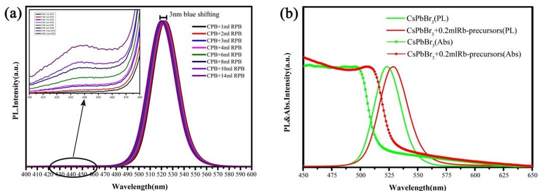
Figure.5s Quantum dots hybrid spectroscopy. (a) The photoluminescence spectra of CsPbBr<sub>3</sub> (CPB) mixed with RbPbBr<sub>3</sub> (RPB); (b) The photoluminescence spectra of CsPbBr<sub>3</sub> mixed with Rb-precursors.
