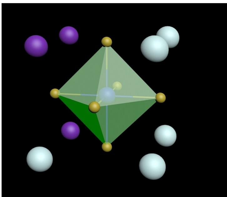
Figure.1s A schematic of the [PbBr<sub>6</sub>] octahedron and Pb-Br bonds in the unit cell of Rb<sub>x</sub>Cs<sub>1-x</sub>PbBr<sub>3</sub> with pm-3m space group.
