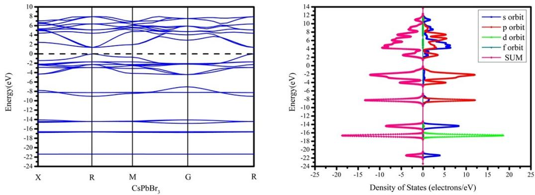
Figure.4s(c) The band structure and DOS of CsPbBr<sub>3</sub> crystal structure with pm-3m space group.
