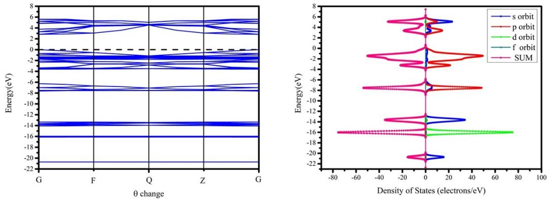
Figure.4s(b) The band structure and DOS of crystal structure with in-plane Pb-Br-Pb bond angle  $\theta$  change.
