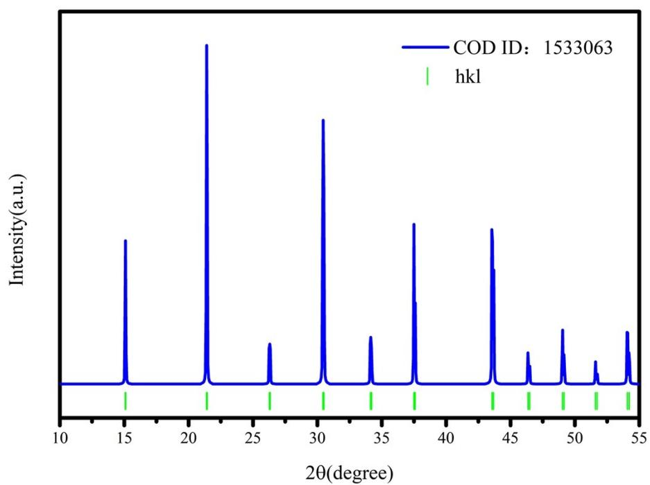
Figure.2s The calculated XRD spectrum of CsPbBr<sub>3</sub> with pm-3m space group.
