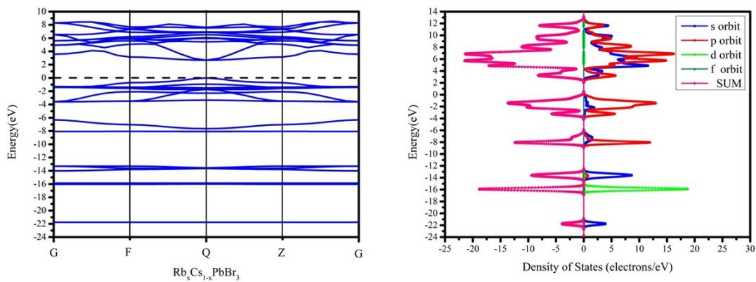
Figure.4s(d) The band structure and DOS of Rb<sub>x</sub>Cs<sub>1-x</sub>PbBr<sub>3</sub> crystal structure with pm-3m space group.
