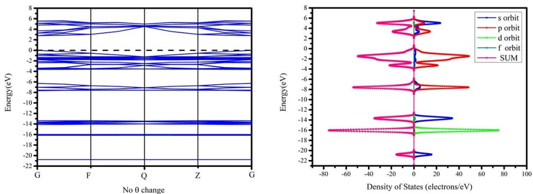
Figure.4s(a) The band structure and DOS of the initial crystal structure.
