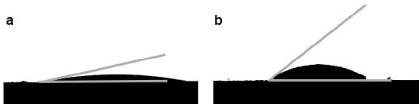
**Figure S10** | The contact angle of PMAG(a) and PMAG after electron beam treatment(b).
