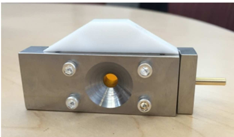
Fig S4: Static reaction cell used for longer time experiments.
