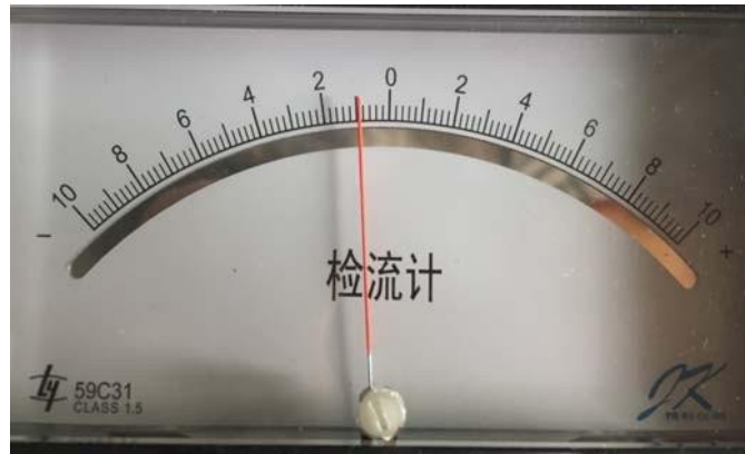
Fig. S14. Image of galvanometer when measuring the net current of h-BN:Mg monolayer with single probe rectification method. The negative net current confirms the p-type conductivity of h-BN:Mg.
