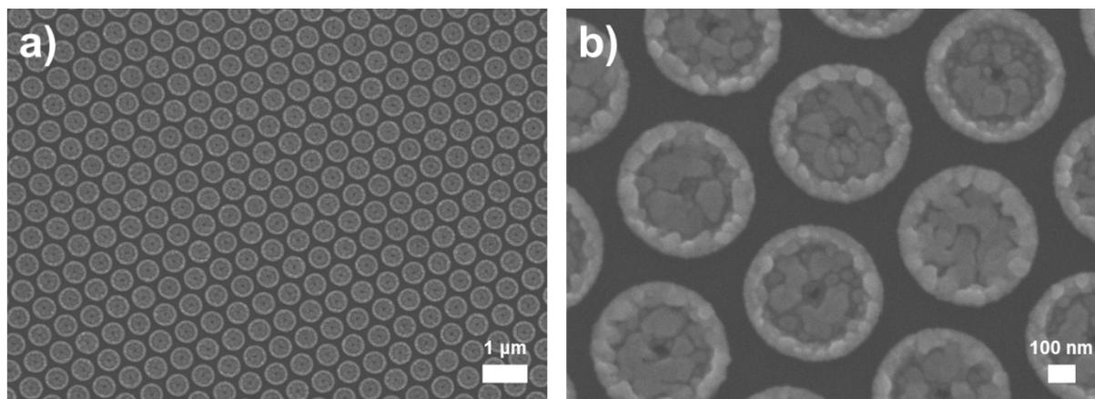
**Figure S3.** a) SEM image of SGB synthesized at an overpotential of  $-4.0$  V vs Ag/AgCl as a reference electrode and b) its magnified image.
