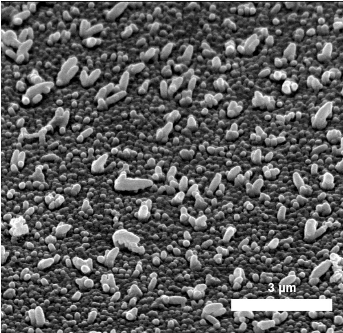
**Figure S12.** Representative SEM image of silver nanostructures grown without NBs.
