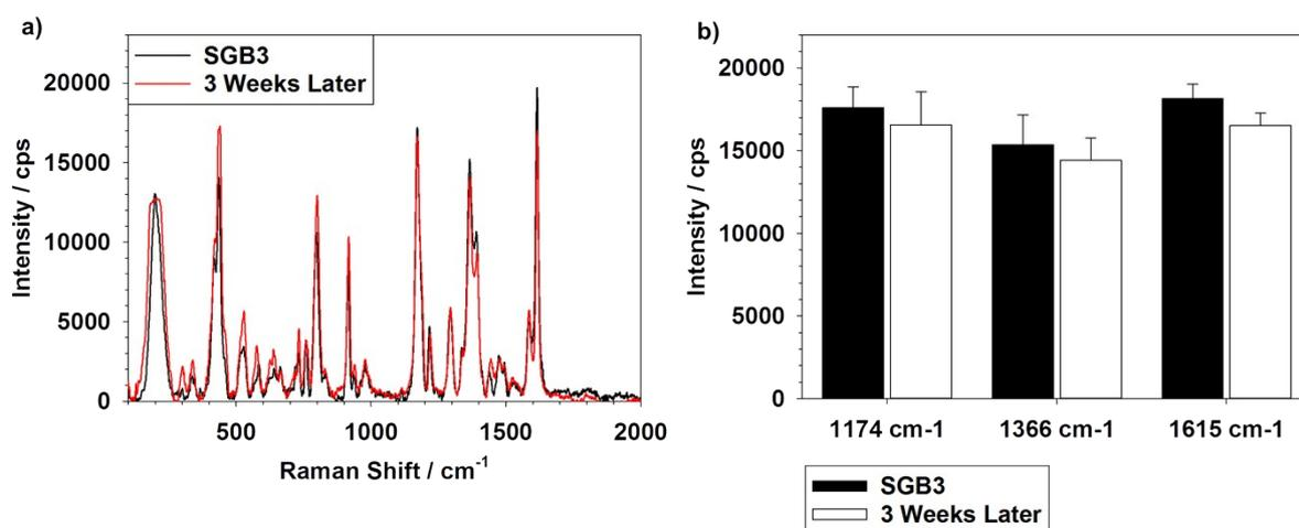
**Figure S15.** Time-dependent stability of SGB3. After synthesis, SGB3 was stored in the desiccator at room temperature and MGITC was used to obtain the SERS signal.
