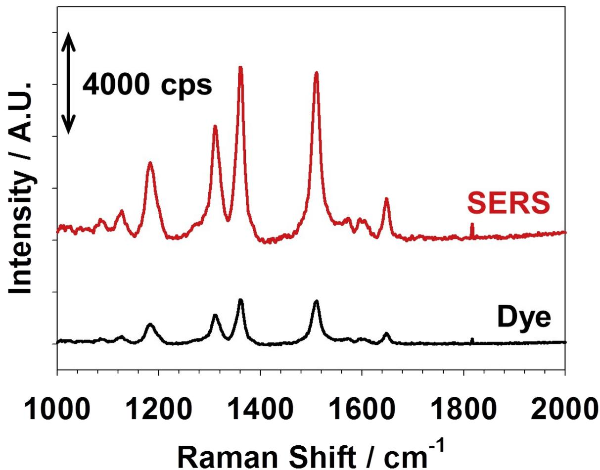
**Figure S16.** SERS spectra of rhodamine 6G adsorbed on a SGB3 SERS substrate and on a planar Si surface. The intensity ratio of the two spectra implies an enhancement factor of  $\sim 10^9$ .
