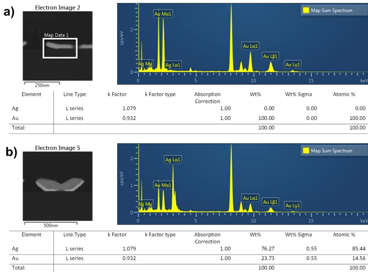
**Figure S10.** EDS spectra and calculated atomic ratios of Ag and Au in a) NB and b) SGB3.
