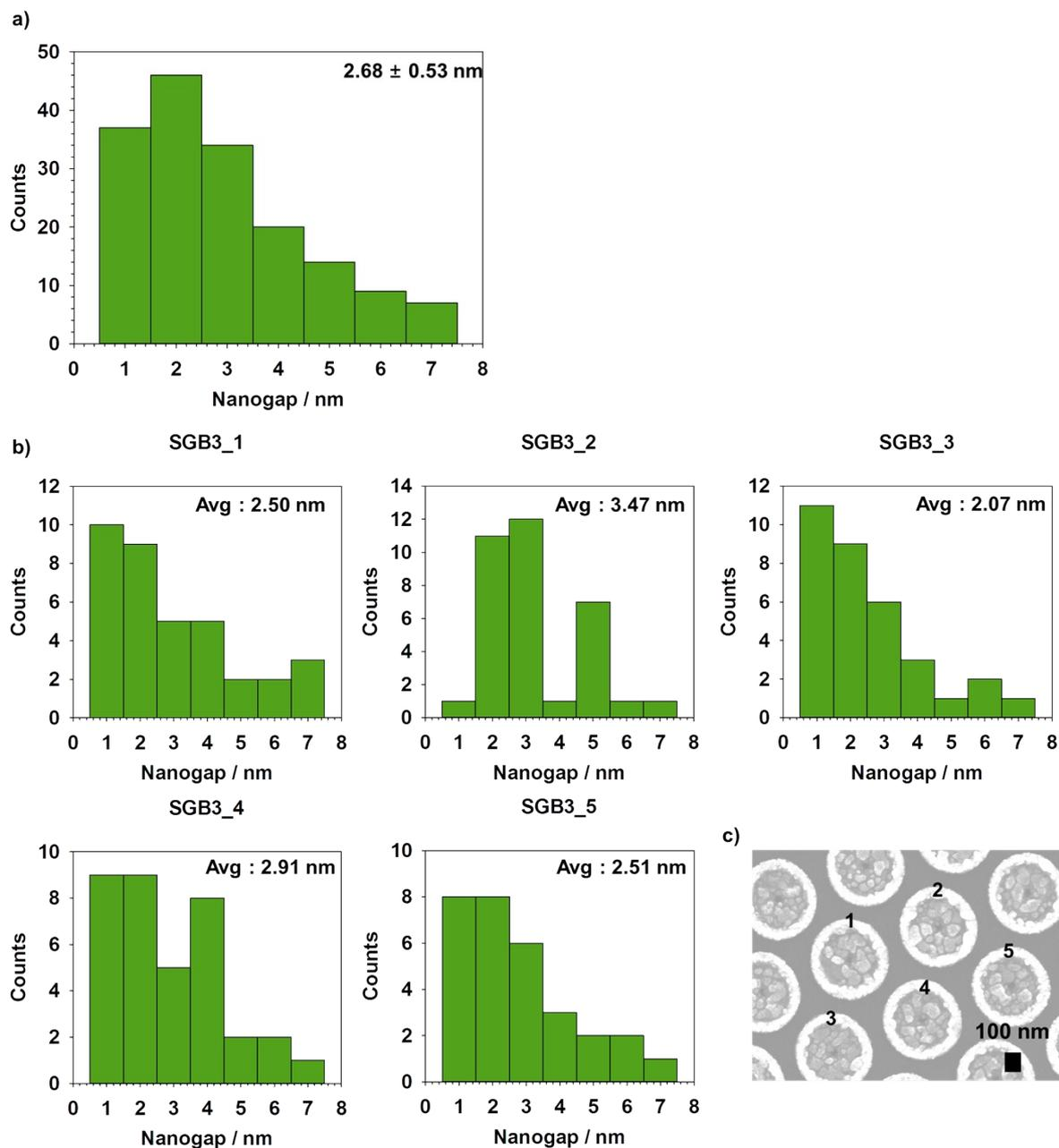
**Figure S1.** a) Nanogap distribution in five SGB3 and b) nanogap distribution in each SGB3 sample. c) SEM images of SGB3 with optimized brightness and saturation for correct analysis. Nanogaps are measured by ImageJ program.
