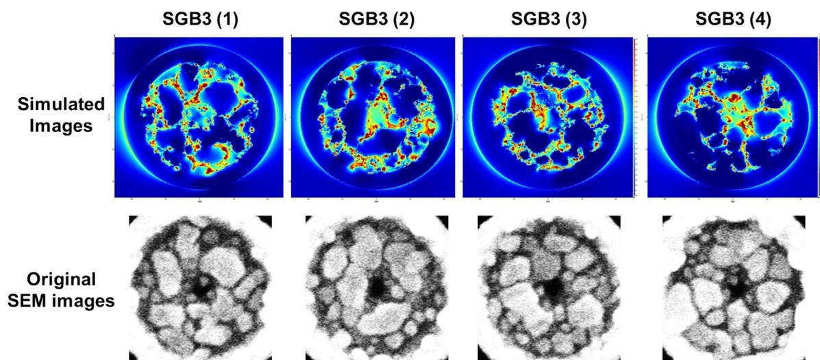
**Figure S17.** FDTD (Finite Difference Time Domain)-simulated EM field distributions of SGB3 and their original SEM images.
