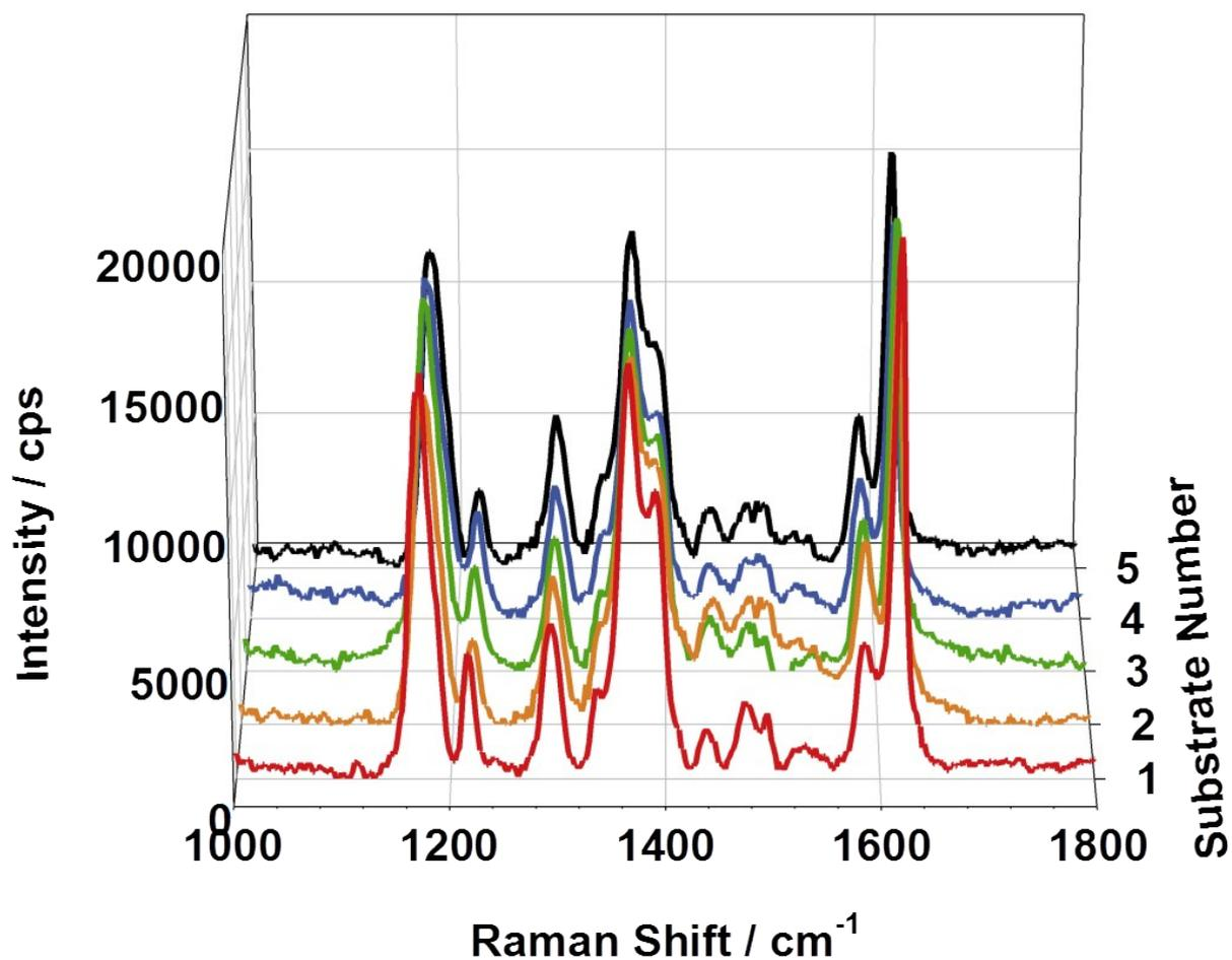
**Figure S14.** Substrate-to-substrate uniformity of SERS spectra under 633 nm laser irradiation of various SGB3 from 5 different batches after  $10^{-7}$  M of MGITC treatment.
