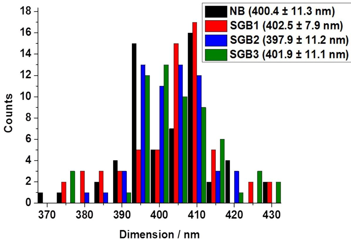
**Figure S2.** Size distribution of NBs before and after silver nanostructure deposition. The dimensions of NBs in the SEM images (Figure 1) are analyzed by ImageJ program.
