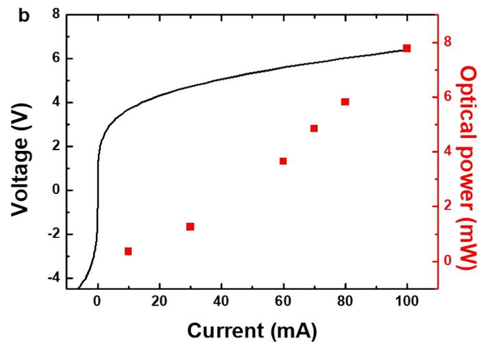
**Figure S4.** (a) Schematic representation of fabrication sequence for DRS LED devices. (b) The light power-current-voltage (L-I-V) characteristics of DRS LED devices. A black solid line is I-V curve and the red squares indicate optical output power at each applied current, respectively.
