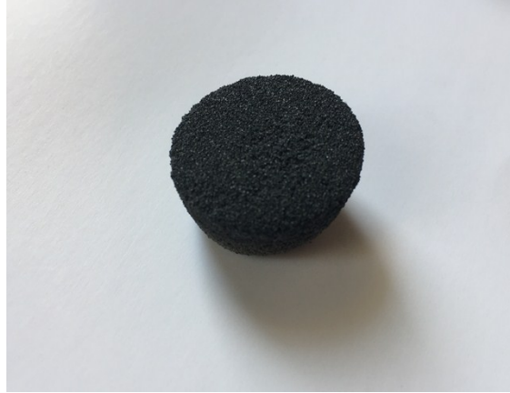
Fig. S1 Digital picture of the mixture ( m_{\text{B4C}}/m_{\text{W}}=1:60 ) after the discharge treatment at 870 °C for 40 min.
