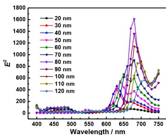
**Fig. S3** LSPR responses for different tip radius illuminated along the tip axis
