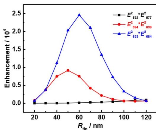
**Fig. S4** The dependence of TERS enhancement on the tip radius at three wavelengths of 532, 594, and 633 nm.
