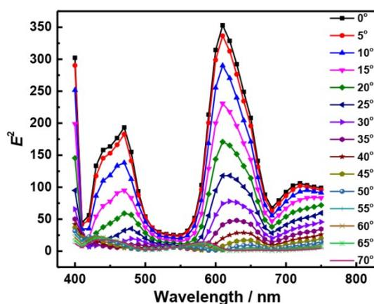
**Fig. S2** Angle dependence of LSPR response for a tip radius of 80 nm
