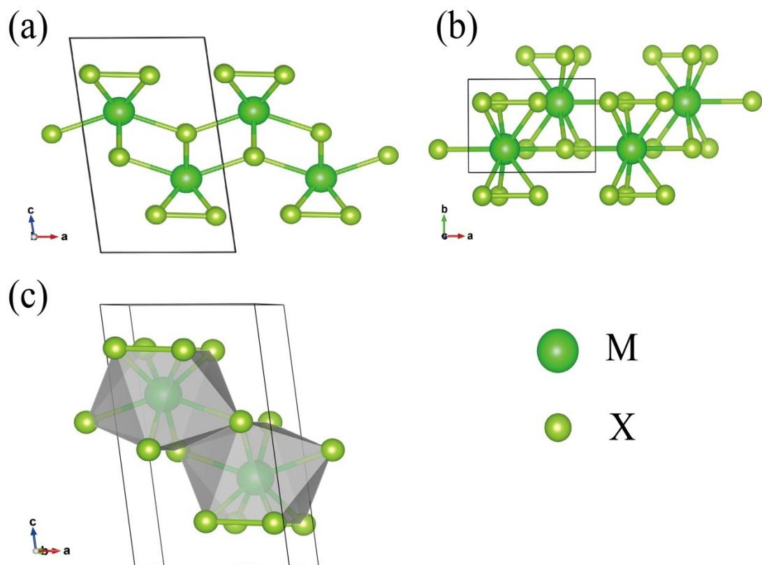
**Fig.S2** (a) Side view of  $\text{MX}_3$ ; (b) Top view of  $\text{MX}_3$ ; (c) The unit cell of  $\text{MX}_3$  structure
