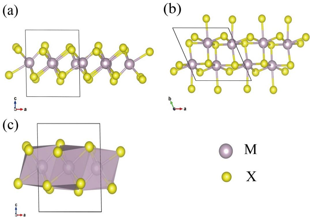
**Fig.S1** (a) Side view of  $\text{MX}_2$ ; (b) Top view of  $\text{MX}_2$ ; (c) The unit cell of  $\text{MX}_2$  structure and the yellow represent chalcogen atoms and purple represent transition metal atoms.
