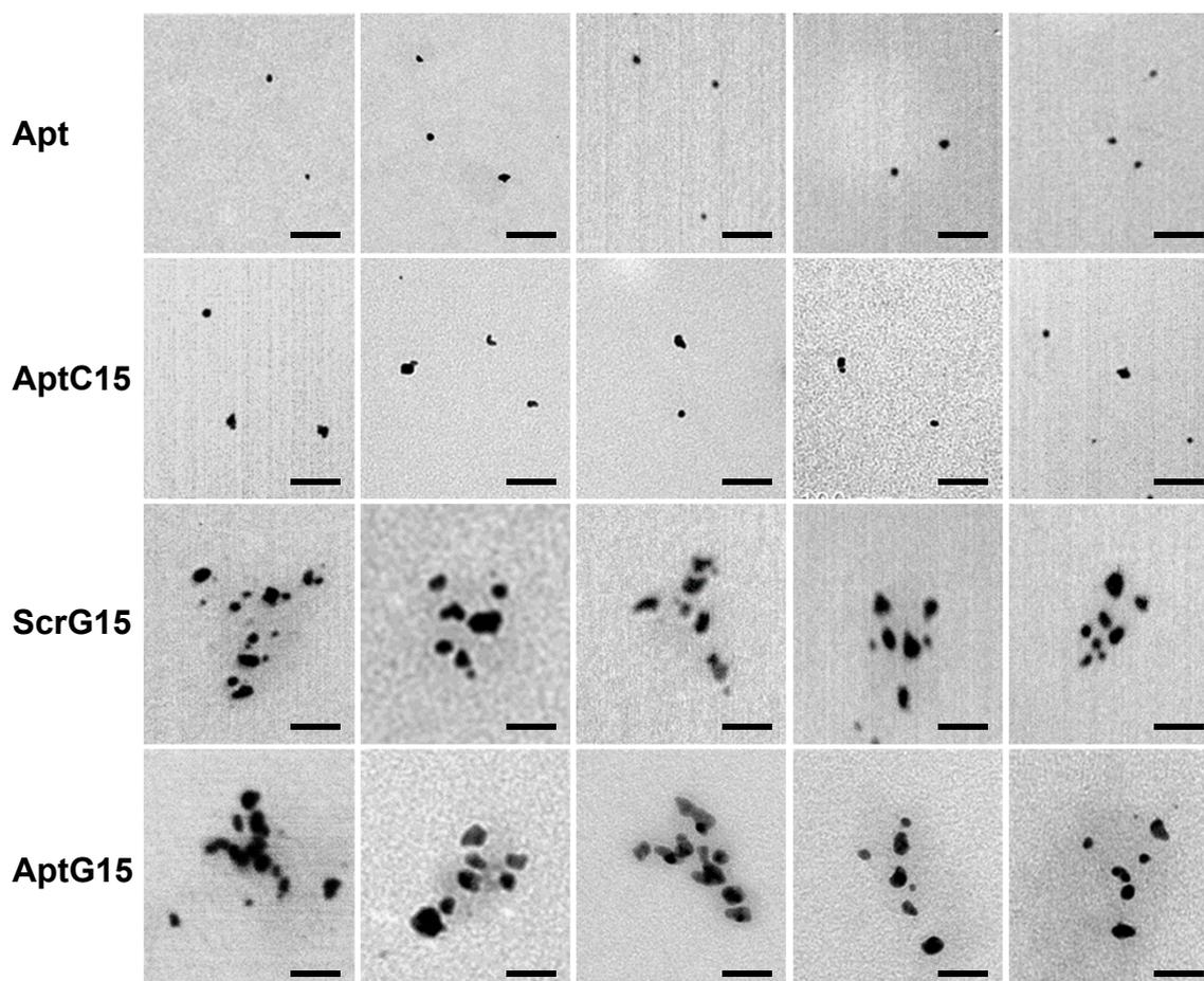
**Supplementary Figure 1. The morphologies of gold-incorporated DNA nanostructures.** For transmission electron microscopy (TEM) imaging, chloroauric acid was added to DNA-based nanostructures for 1 h at room temperature. After removal of free chloroauric acid following reduction, the gold-loaded DNA nanostructures were visualized by TEM. For each condition, five pictures were presented. Scale bar: 25 nm.
