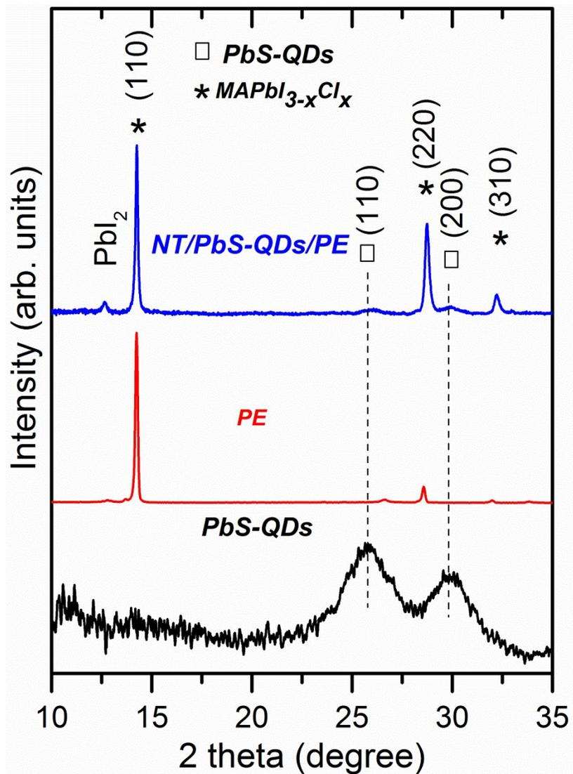
**Fig. S3** X-ray diffraction measurements of the PbS-QDs, the MAPbI<sub>3-x</sub>Cl<sub>x</sub> and the SWCNT/PbS-QDs/MAPbI<sub>3-x</sub>Cl<sub>x</sub>. The size of PbS-QDs used in these measurements is around 2.88 nm.
