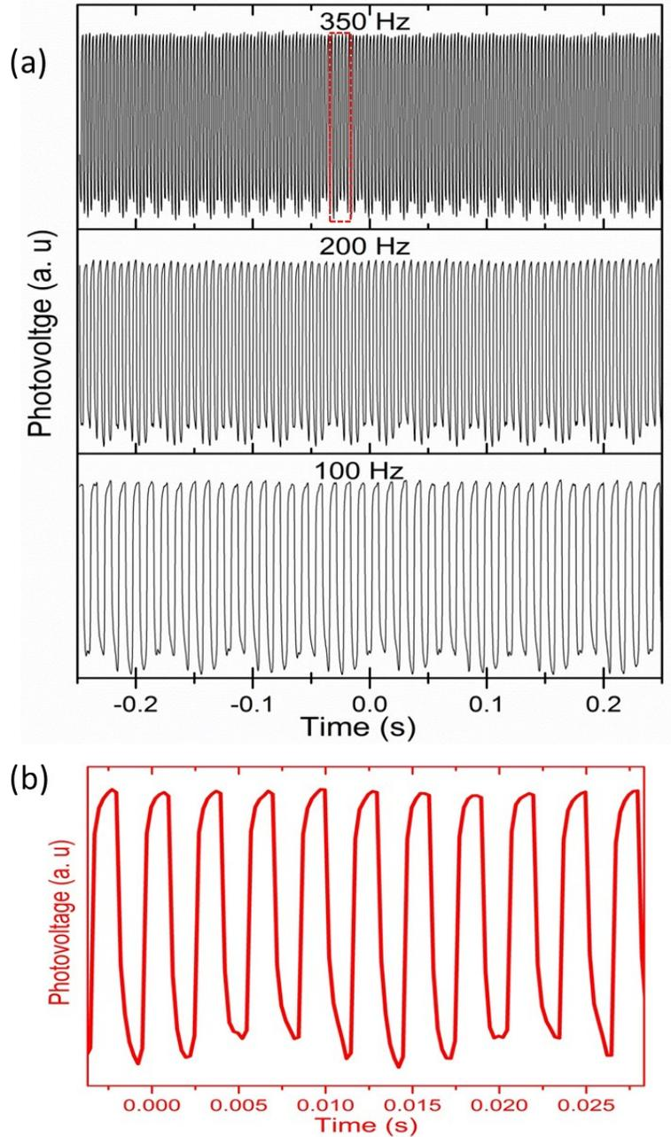
**Fig. S8** a) Typical time response measurements of the NT/PbS-4.35nm/PE device measured at 2 V and under repetitive on/off cycles, using a chopper at different frequencies 100 Hz, 200 Hz and 350 Hz. The illumination was a continuous laser at 532 nm. b) Zoom-in of the red rectangle in upper of (a).
