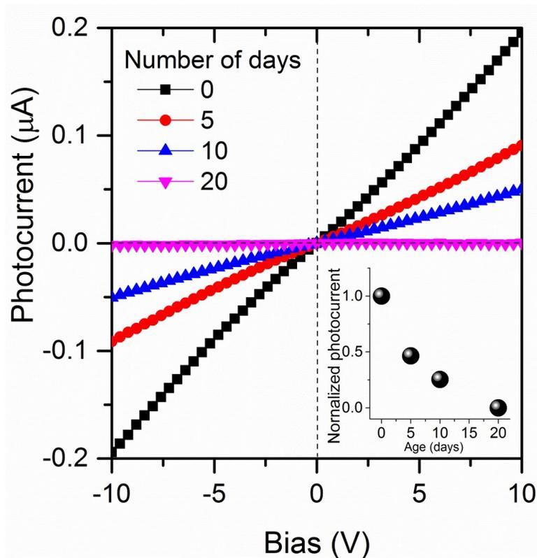
**Fig. S7.** Typical variation of the photocurrent over 20 days in ambient air. The bottom inset shows the normalized variation of the photocurrent.
