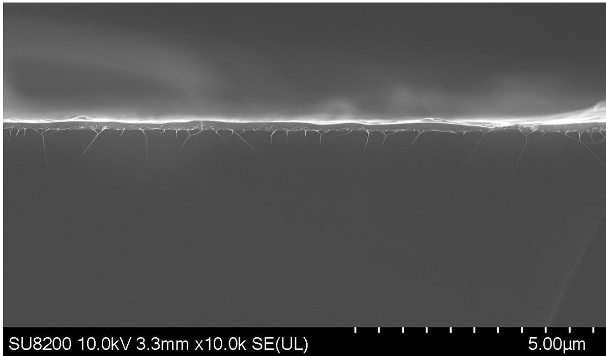
**Fig. S2** Cross sectional SEM image of SWCNT/PbS-QDs/perovskite at low magnification, showing the uniformity of the hybrid film. The SWCNTs are deposited by spray-coating, the PbS-QDs are deposited by dip-coating and the perovskites are deposited by spin-coating.
