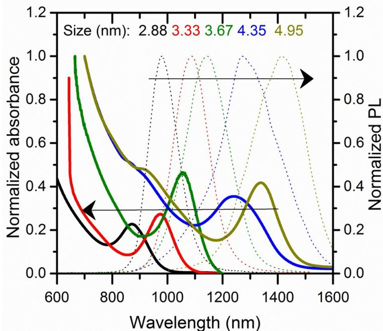
**Fig. S1** Normalized absorption and photoluminescence of the PbS-QDs of different sizes used in this work. The estimation of the QDs sizes were determined using data reported by Sablon et al<sup>1</sup>.
