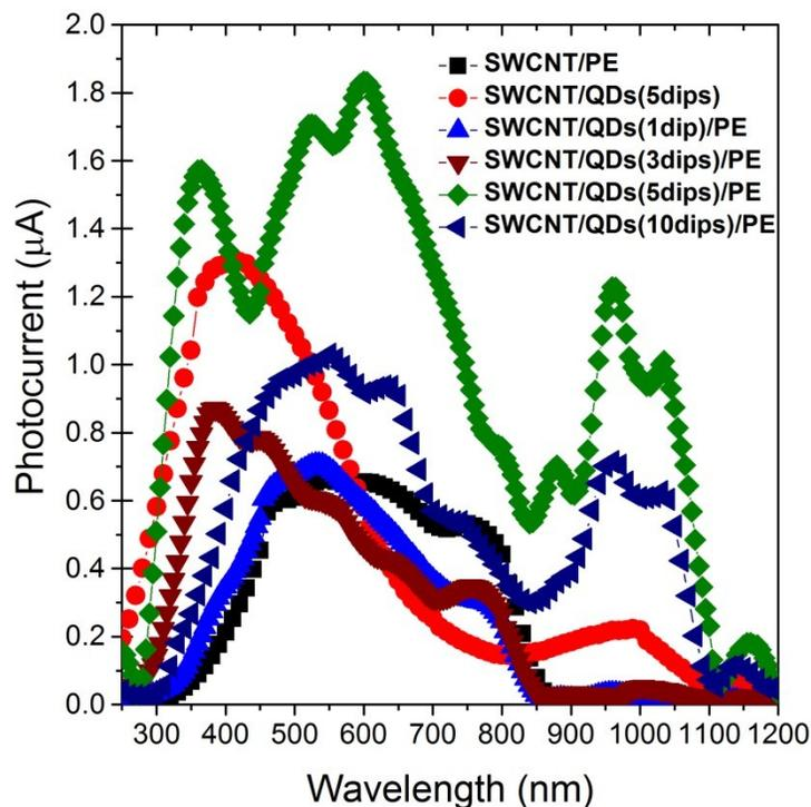
**Fig. S4** Optimization of the number of dips of PbS-QDs through the photocurrent spectrum measurements. The addition of PbS-QDs as another sensitizer shows additional responses in the UV and the NIR regions. The samples made with 5 dips exhibits the highest response both in the NIR and the visible. The size of PbS-QDs used in these measurements is around 2.88 nm.
