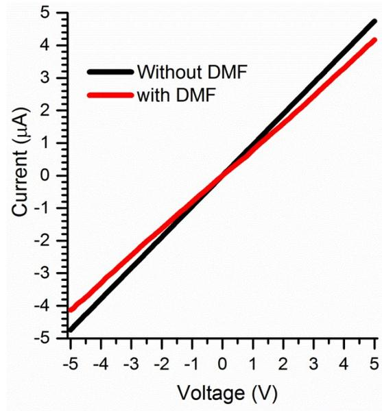
**Fig. S6.** I-V curves of a given SWCNT film before and after an addition of DMF, demonstrating that the lower dark current from the SWCNT/PbS-QDs/PE device is due to the DMF solvent that is used in the synthesis of the perovskite solution.
