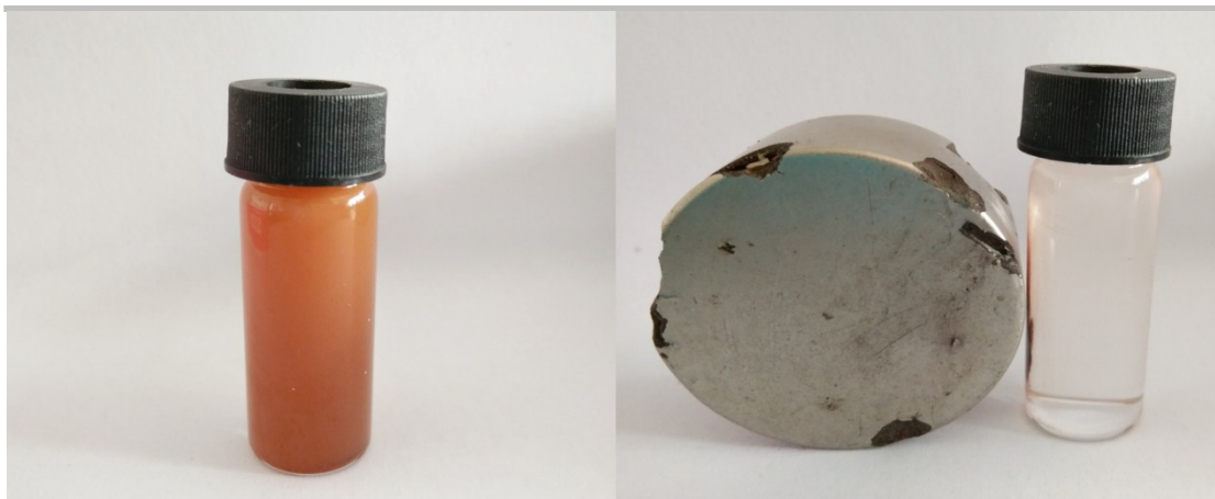
Fig S3. Pictures of FSAu@mSiO 2 @L-Cys nanoparticles (a) dispersed in distilled water; (b) separated from distilled water by a magnet after 30 seconds.
