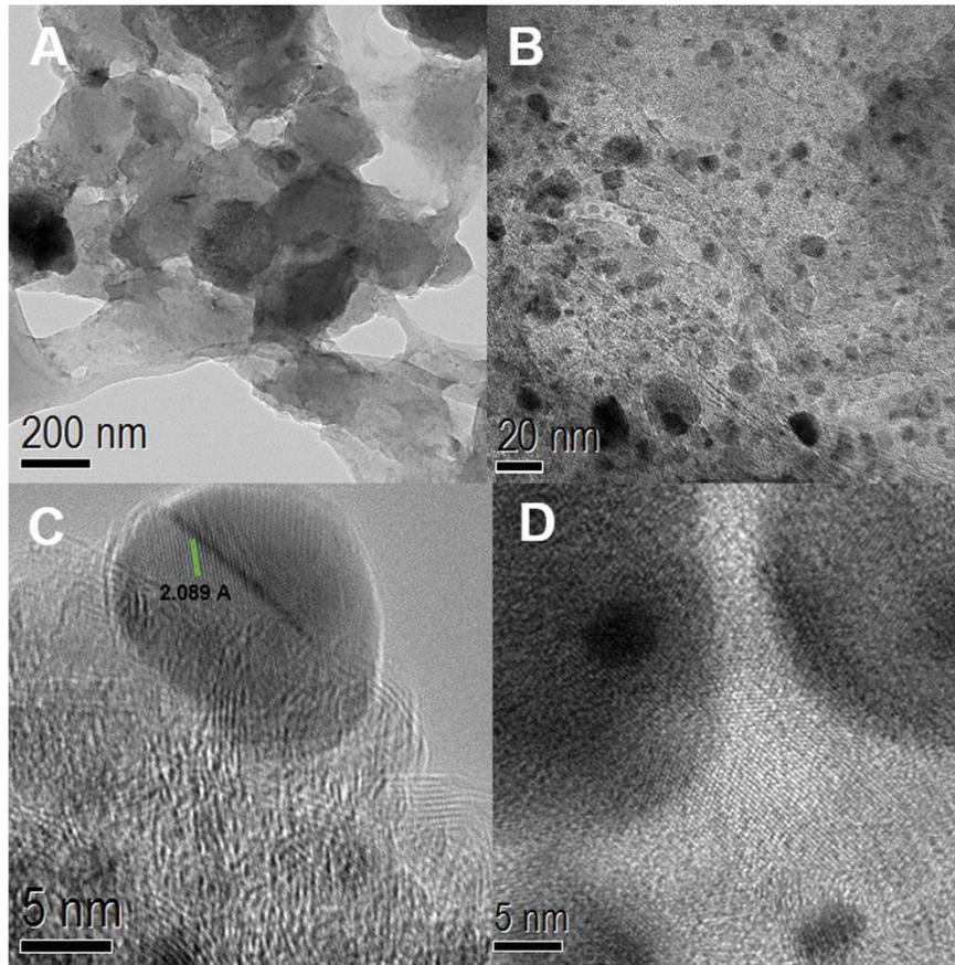
**Figure S6** (A) and (B) TEM images, and (C) and (D) HRTEM images of ENPS electrode after first full discharge.
