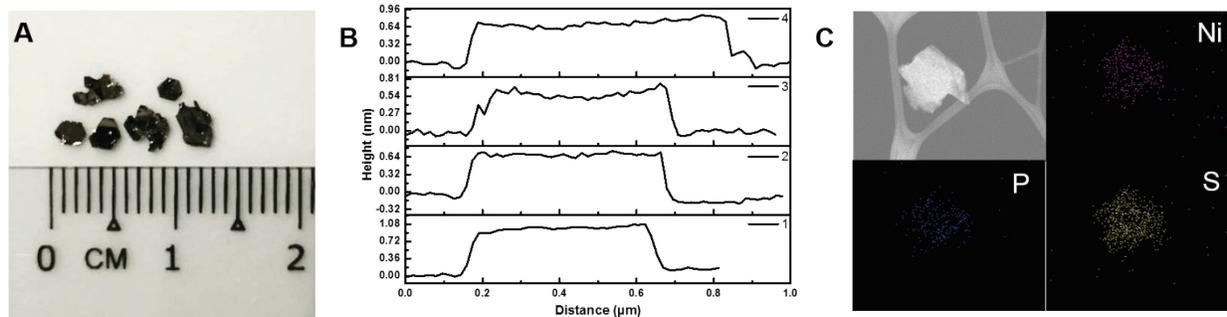
**Figure S3** (A) Hexagonal bulk crystals of NiPS<sub>3</sub>, (B) AFM height profiles of ENPS nanosheets in Figure 3 and (C) Elemental mapping of ENPS nanosheets.
