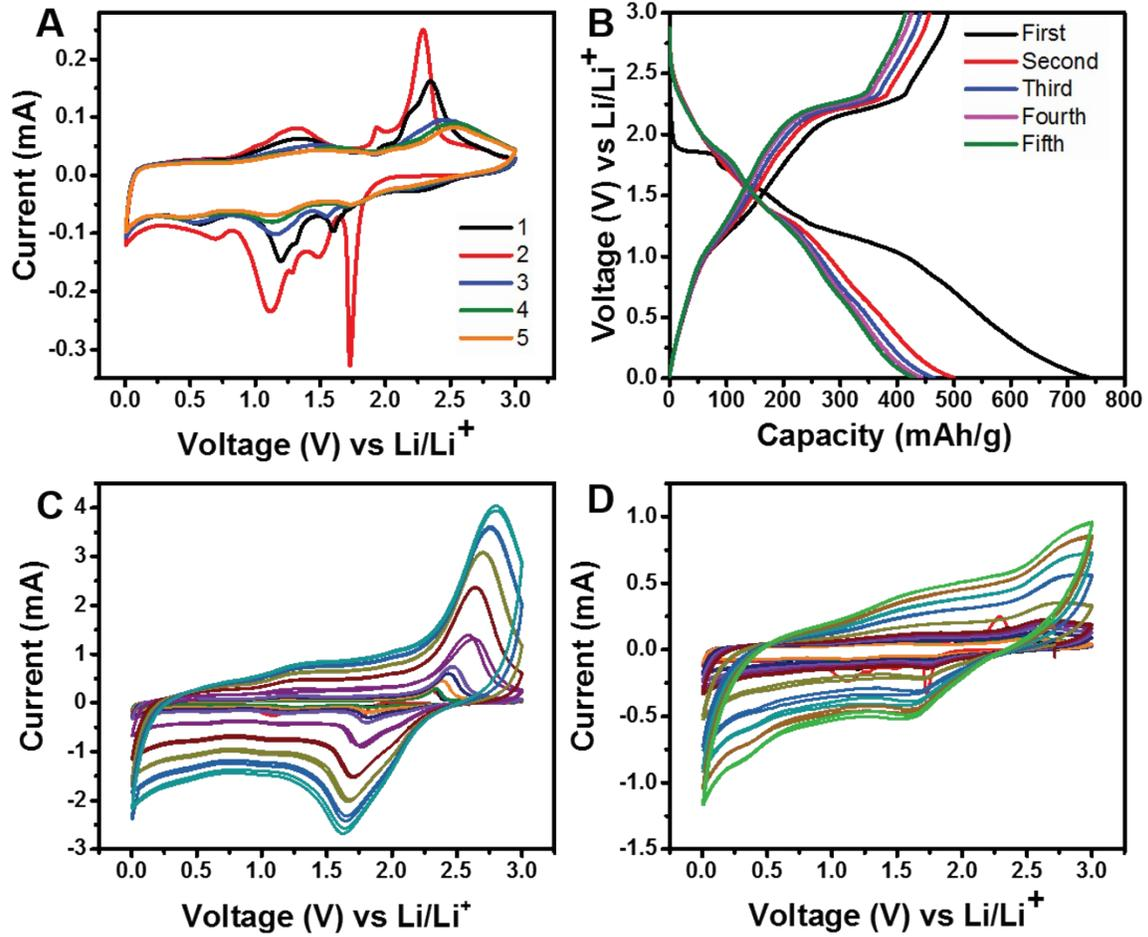
**Figure S5** (A) First five CV cycles of BNPS at  $0.1 \text{ mV s}^{-1}$ , (B) First five charge-discharge cycles of BNPS at  $0.1 \text{ A g}^{-1}$ , (C) CV cycles of ENPS at various rates ( $0.1 - 5 \text{ mVs}^{-1}$ ) and (D) CV cycles of BNPS at various rates ( $0.1 - 5 \text{ mVs}^{-1}$ ).
