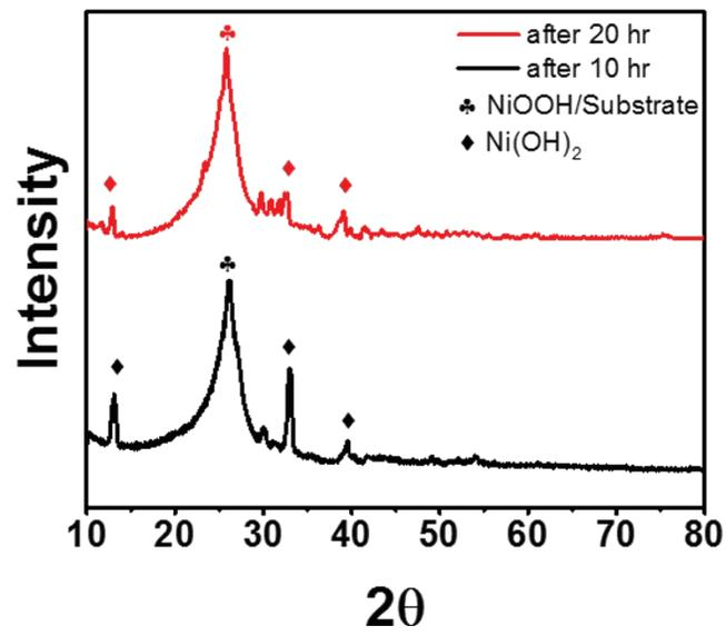
Figure S9 XRD patterns of ENPS after OER durability testing.
