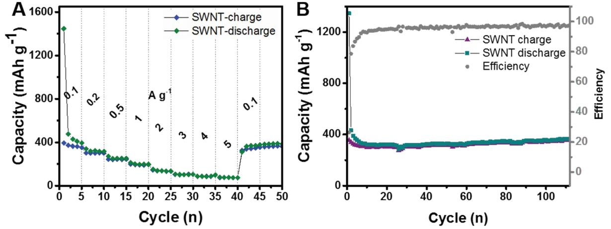
Figure S2 (A) Charge and discharge specific capacities at different current densities of single walled carbon nanotubes and (B) Cycling capacity of single walled carbon nanotubes at 0.1 A g<sup>-1</sup>.
