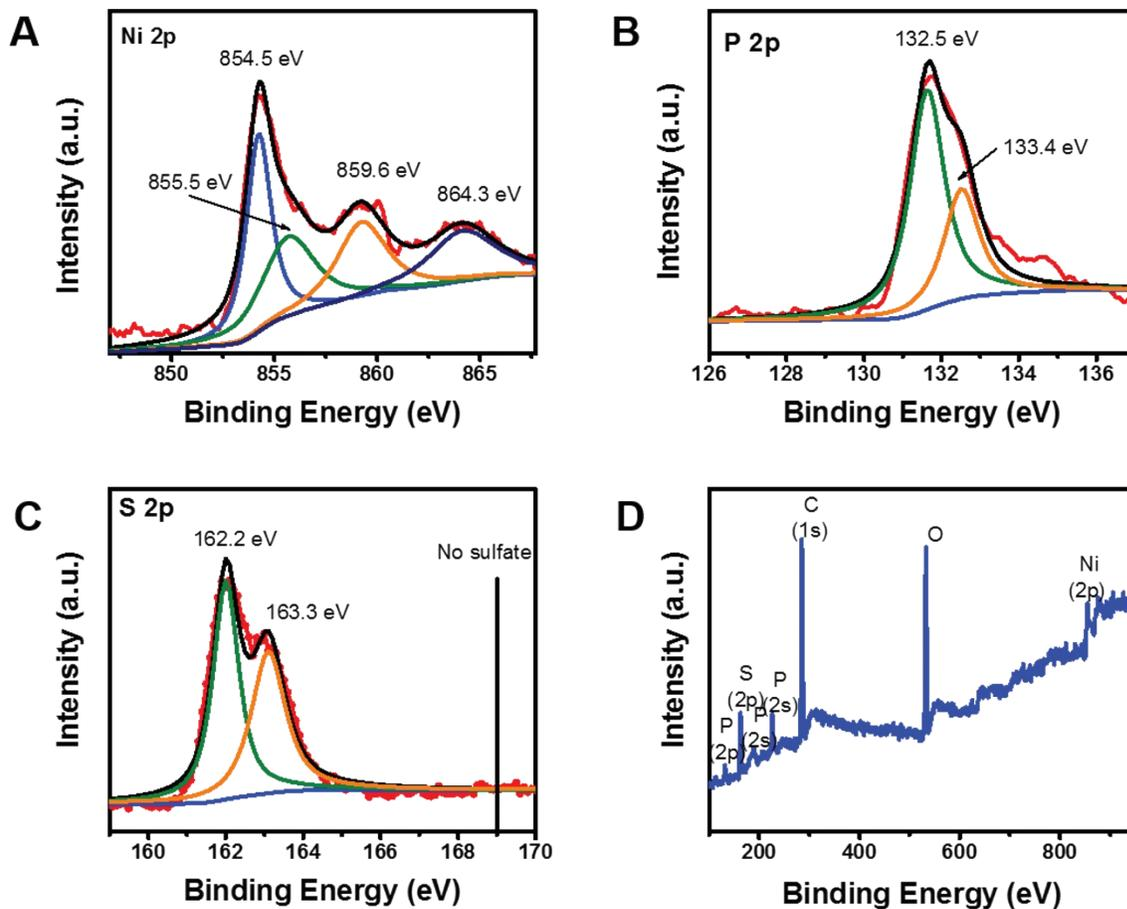
Figure S4 XPS spectra of (A) Ni 2p, (B) P 2p, (C) S 2p, and (D) Survey XPS spectrum.
