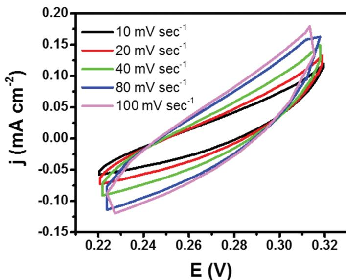
Figure S7 CV in the range of 0.22 V - 0.32 V for the calculation of ECSA of ENPS.
