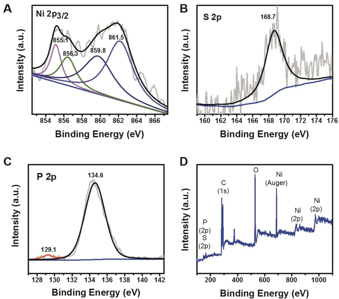
Figure S8 XPS spectra of (A) Ni 2p<sub>3/2</sub>, (B) S 2p, (C) P 2p and (D) Survey XPS spectrum of ENPS after OER.
