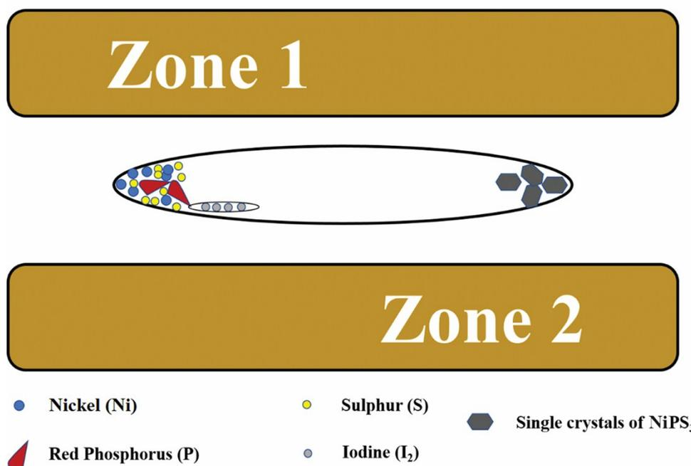
Figure S1 Schematic of preparation of NiPS<sub>3</sub> bulk crystal.
