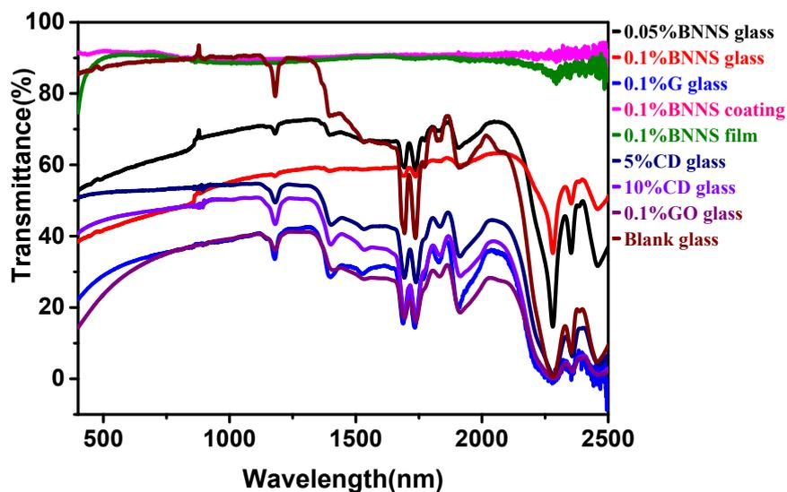
Figure S3. Transmittance spectra of blank and hybrid Ormosil gel glasses solid structures (~0.1 wt%): blank gel glass; 0.05 wt% BNNs doped glass, 0.1 wt% BNNs doped glass, 0.1 wt% BNNs gel coating (on glass) and 0.1 wt% BNNs self-healing film; 5 wt% and 10 wt% carbon dot (CD) doped gel glass; and 0.1 wt% graphene (G) and 0.1 wt% graphene oxide (GO) doped glass, respectively.
