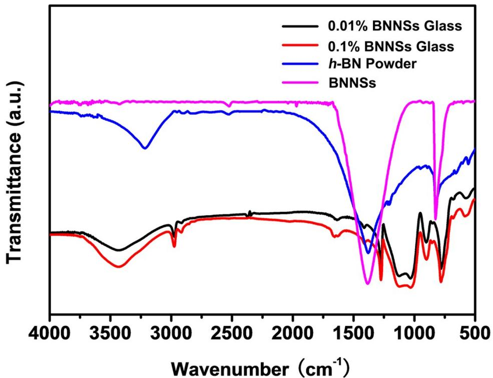
Figure S1. FTIR spectra of h-BN raw materials (blue line), BNNs (pink line), 0.01% BNNs doped glass (black line) and 0.1% BNNs doped glass (red line), respectively.
