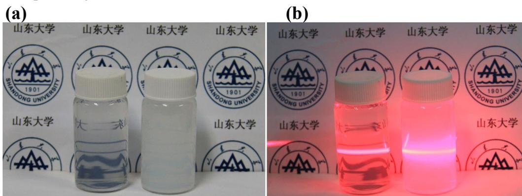
Figure S2. Photograph of BNNs suspension and their Tyndall effects, the solvents of the dispersion from left to right are ethanol and water. (a) h-BN nanosheets dispersions upon visible light (b) Tyndall effects of the nanosheets dispersions, laser light shone from left.
