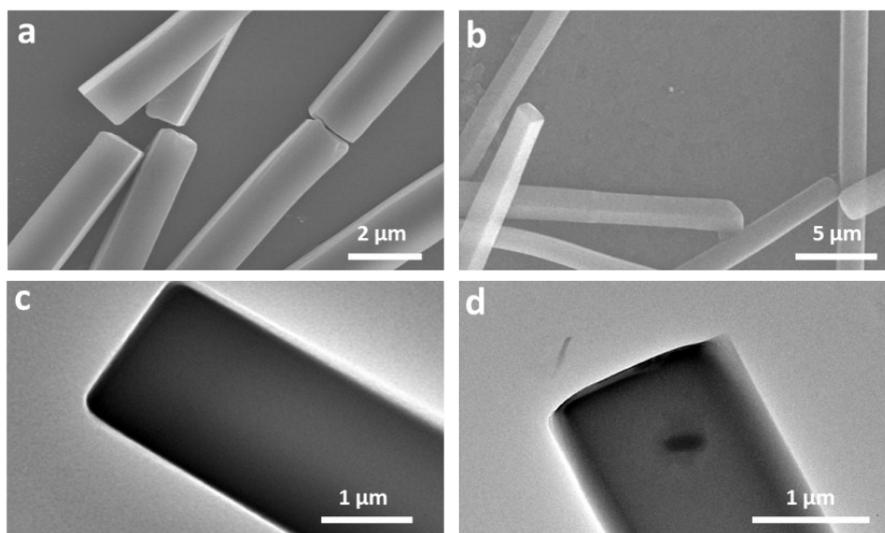
**Figure S4.** (a-b) SEM images and (c-d) TEM images of DMHP organic micro-rods with the flat cross-sectional plane. The scale bars are (a) 2  $\mu\text{m}$ , (b) 5  $\mu\text{m}$  and (c-d) 1  $\mu\text{m}$ , respectively.
