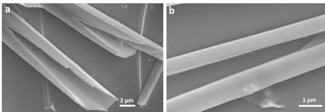
**Figure S9.** SEM images of these cracked DMHP organic micro-tubes. The scale bars are (a) 2 and (b) 1  $\mu\text{m}$ , respectively.
