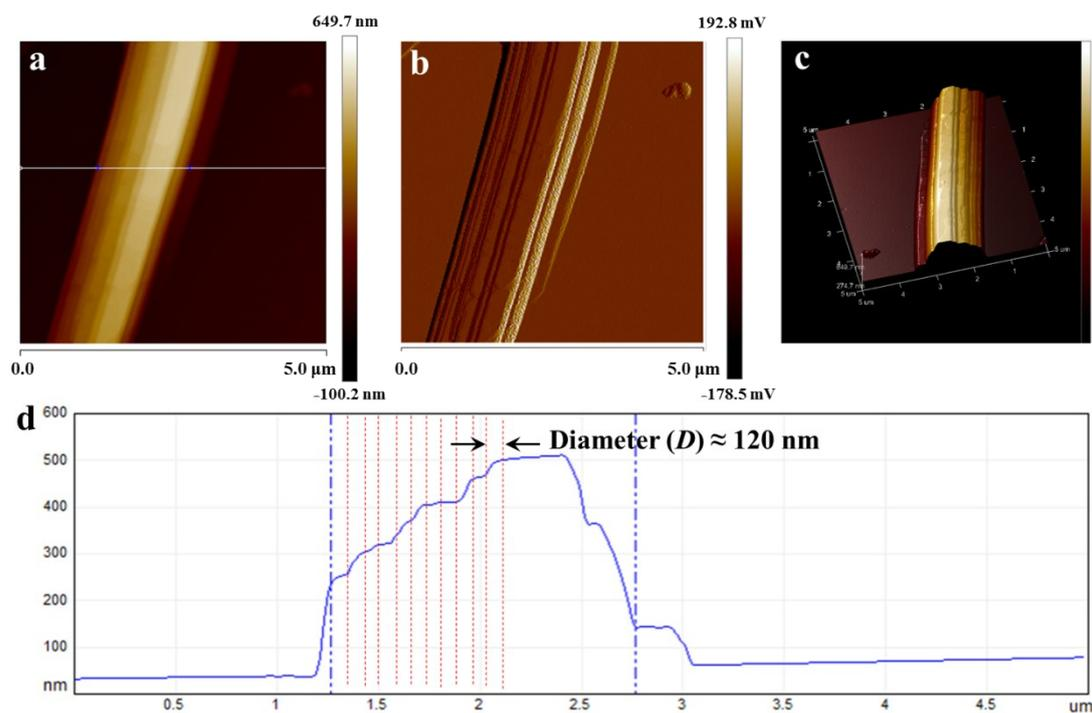
**Figure S13.** (a-c) AFM images of the typical DMHP organic bouquet-like bundle. (d) The height profile corresponding to the white line in Figure S13a.
