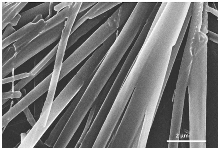
**Figure S10.** SEM image of the bouquet-like bundles of regular and inchoate DMHP organic nanowires with scale bar of 2  $\mu\text{m}$ .
