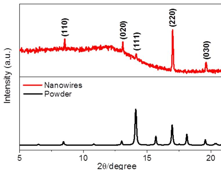
**Figure S15.** X-ray diffraction patterns of these as-prepared organic nanowires (red line, top panel) and simulated powder pattern using Mercury software (black line, bottom panel)
