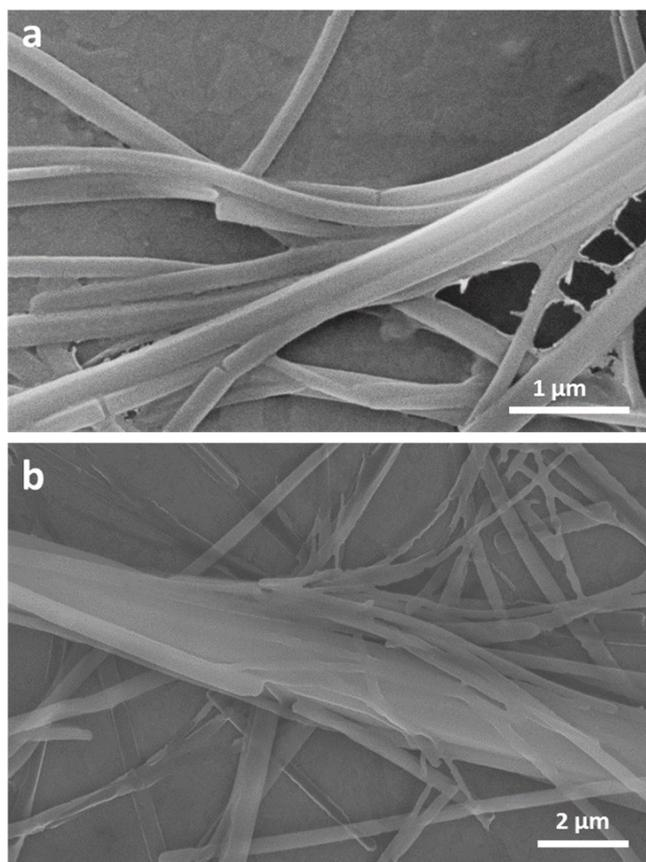
**Figure S12.** SEM images of the DMHP organic bouquet-like bundle with the scale bars of (a) 1 and (b) 2  $\mu\text{m}$ , respectively.
