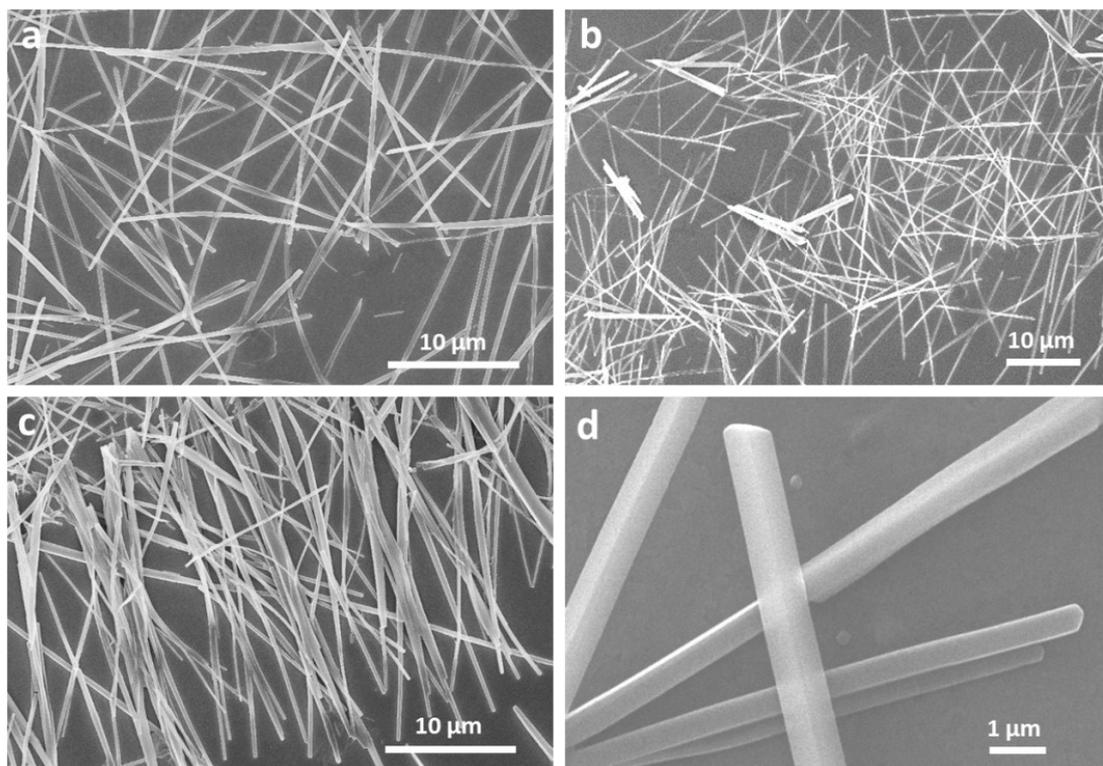
**Figure S8.** SEM images of the DMHP organic micro-rods according to orthogonal solvents of DCM and *n*-hexane with different sampling time: (a) 30 min, (b) 6 hours, (c) and (d) 12 hours. The scale bars are (a-c) 10 and (d) 1  $\mu\text{m}$ , respectively.
