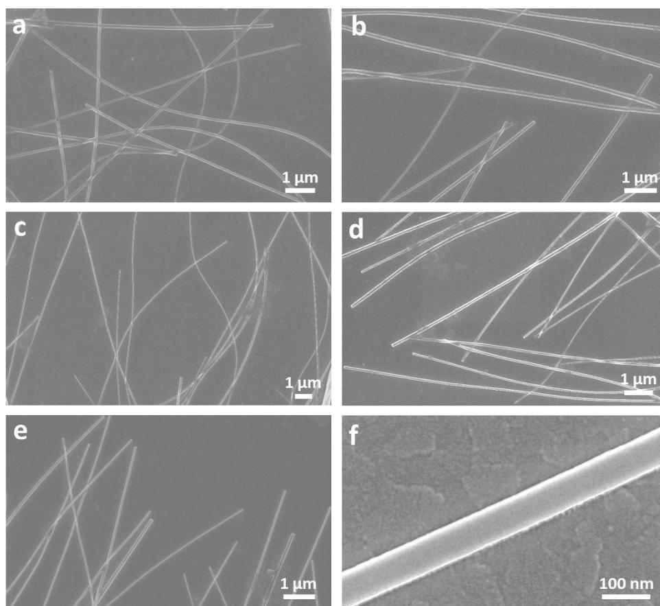
**Figure S14.** SEM images of the DMHP organic nanowires. The scale bars are (a-e) 1  $\mu\text{m}$  and (f) 100 nm, respectively.
