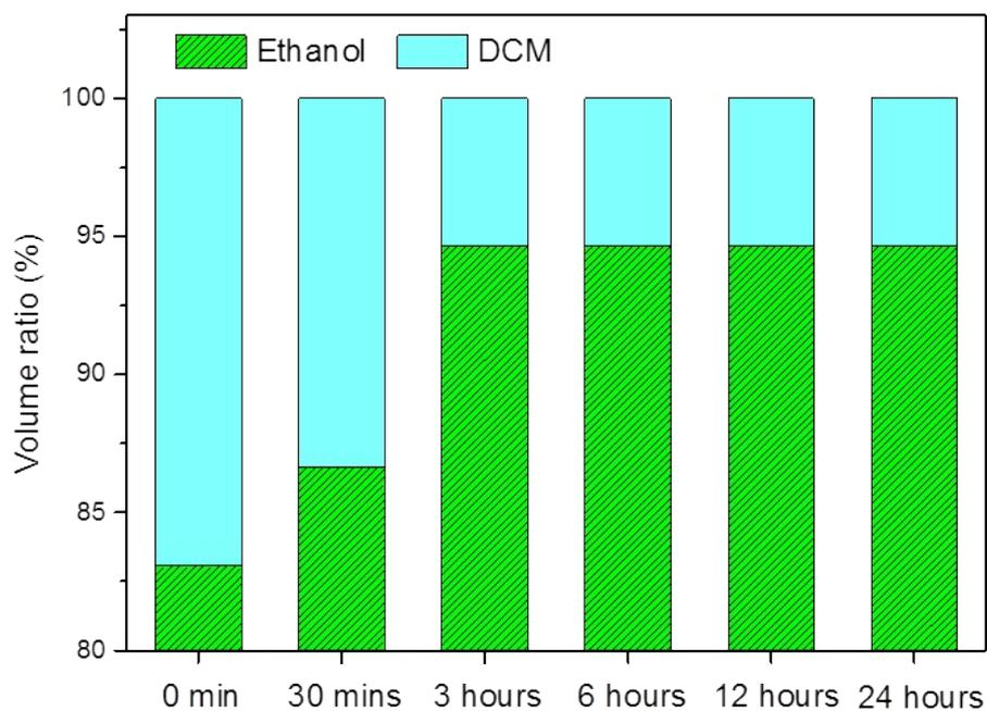
**Figure S6.** The volume ratios of ethanol (DCM) at 0, 0.5, 3, 6, 12, and 24 hours (the mixed solvent system is exposed to the air). And the volume ratio is confirmed by the gas chromatography.
