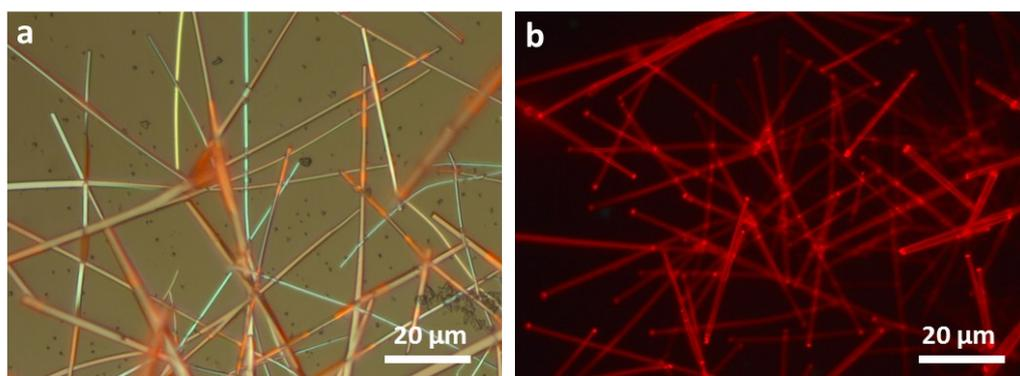
**Figure S3.** (a) The bright optical image of these as-prepared organic microrods at sampling time of 30 minutes. The scale bar is 20 μm. (b) The fluorescence microscopy image of the as-prepared organic microrods (at sampling time of 30 minutes) excited with UV band (330-380 nm) from a mercury lamp. The scale bar is 20 μm.
