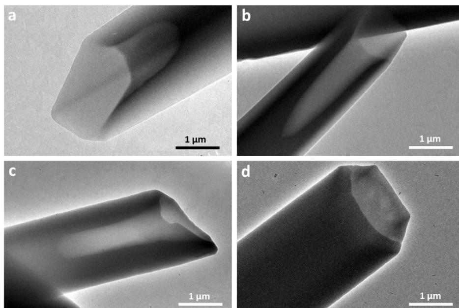
**Figure S5.** TEM images of the DMHP organic micro-rods with hollow structure in the edge. The scale bars are 1  $\mu\text{m}$ .
