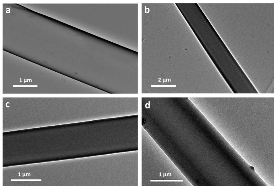
**Figure S7.** TEM image of the DMHP organic micro-tubes. The scale bars of (a, c, d) and (b) are 1 and 2  $\mu\text{m}$ , respectively.
