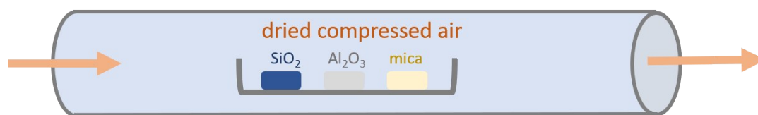
Fig. S1 Schematic diagrams of the thermal annealing equipment setup.
