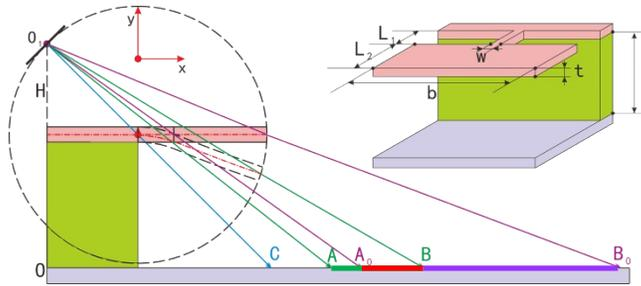
**Figure S1** Simplified geometrical model of the optical projection controllable microweighing sensor.
