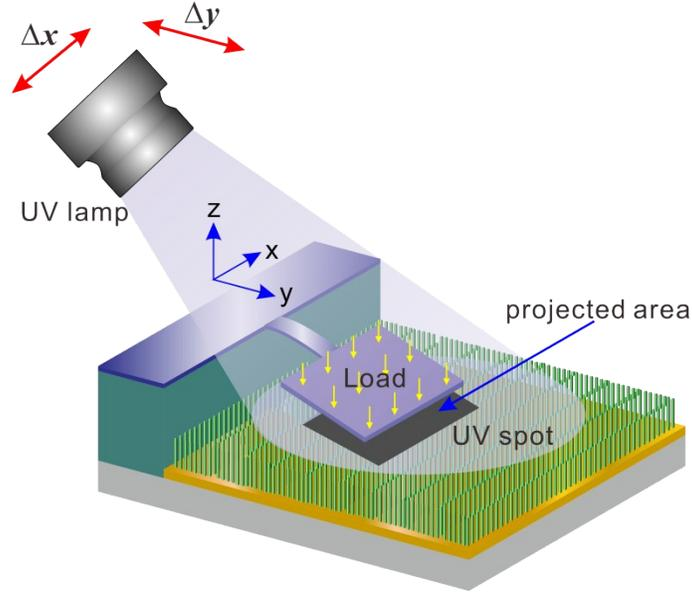
**Figure S3** Schematic illustration of the adjustment of UV light source.
