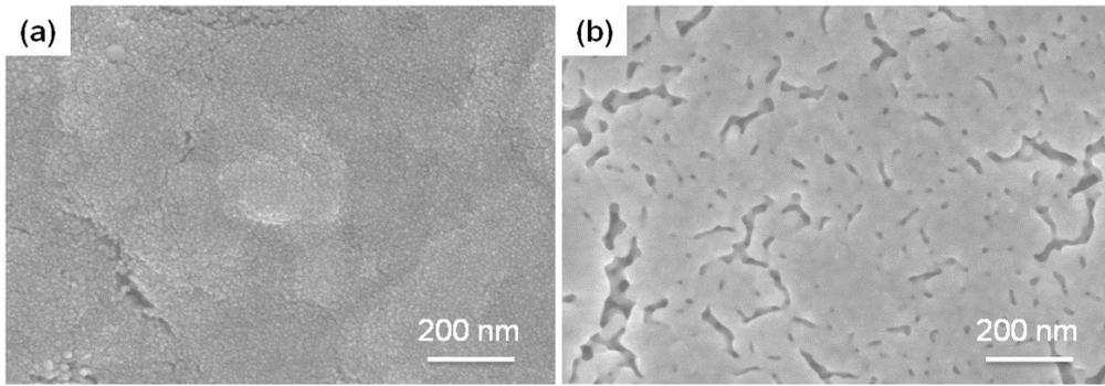
Fig. S6 Microstructures of (a) original Cu-63Ag-100 track and (b) Cu-63Ag-100 track after aging at 80 for 2 h.
