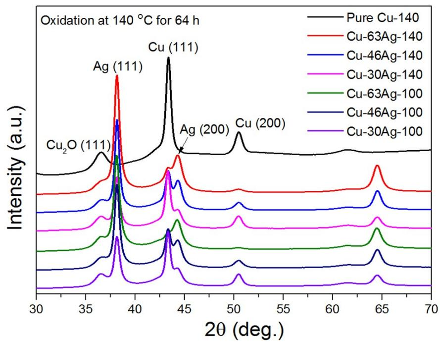
Fig. S7 XRD patterns of printed tracks after oxidation at 140 °C for 64 h.
