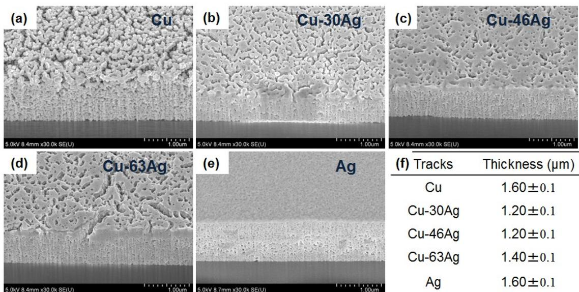
Fig. S2 Thickness measurement of printed tracks based on SEM images. Cross-section images of printed tracks prepared from (a) Cu complex ink, (b) Cu-30Ag complex ink, (c) Cu-46Ag complex, (d) Cu-63Ag complex ink and (e) Ag complex ink; (f) thickness values of printed tracks. The SEM images were taken on an angle of  $30^\circ$ .
