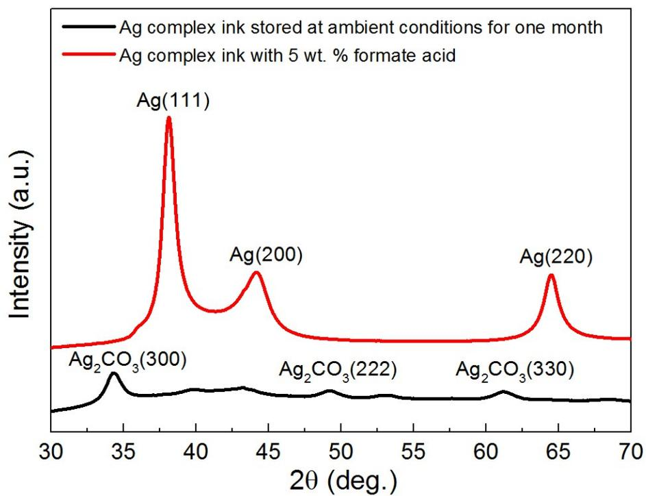
Fig. S4 XRD patterns of Ag complex ink after storage in ambient conditions for one month and Ag complex ink with addition of 5 wt. % formate acid.
