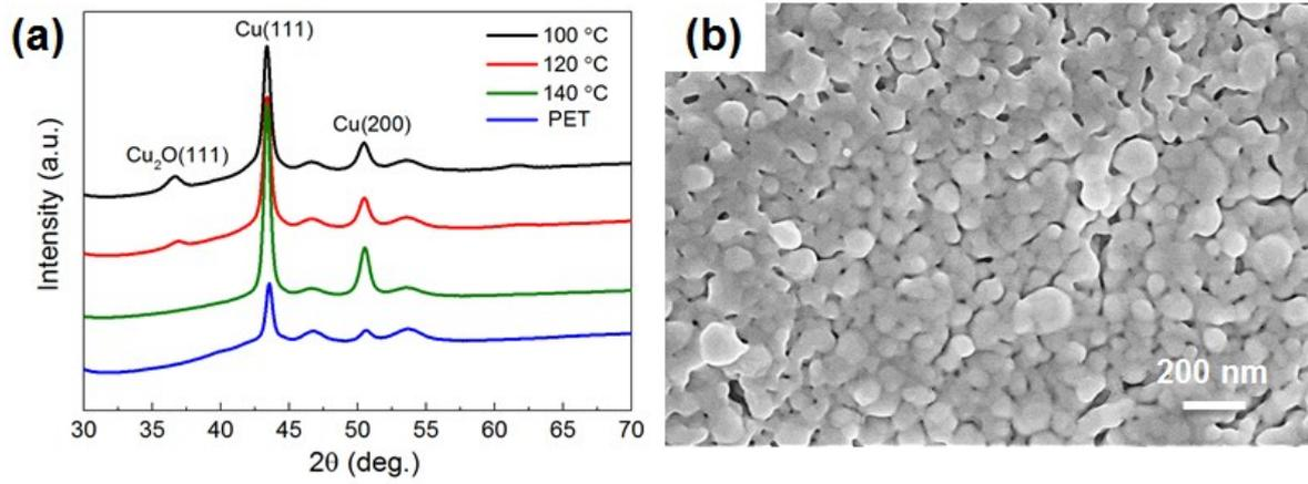
Fig. S3 (a) XRD patterns of Cu track annealed at different temperatures for 30 min and (b) microstructure of Cu track annealed at 140 °C for 30 min.
