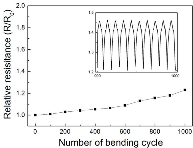
Fig. S8 Change of relative resistance of the Cu-46Ag track during bending test. The bending radius is 7 mm. Inset graph shows the real-time relative resistance during the last ten cycles of bending and releasing process.
