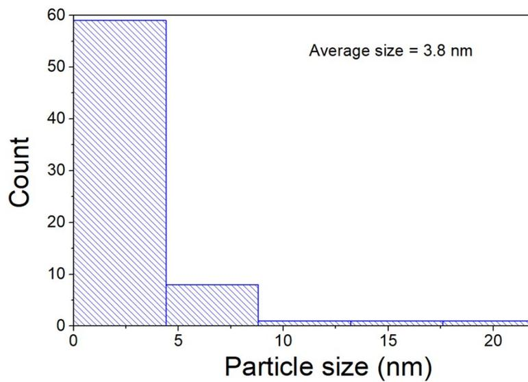
Fig. S5 The distribution of particle size of in-situ formed Ag nanoparticles.
