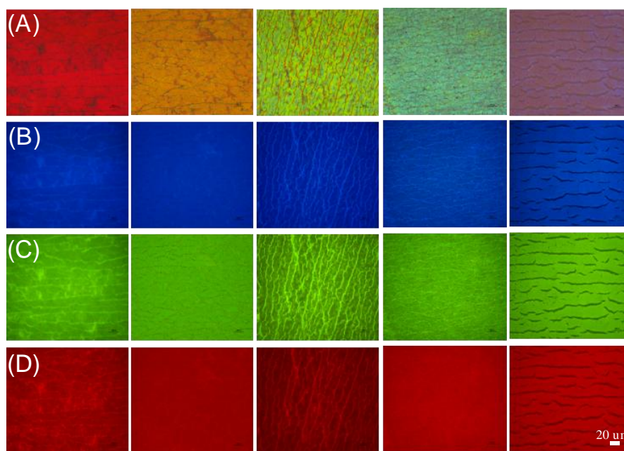
Figure S5. (A) Optical images of SiCDIOs with different bandgaps, such as 675, 610, 542, 517 and 466 nm respectively from left to right. (B-D) The fluorescent images of corresponding samples that being excited at laser of (B) 375, (C) 480 and (D) 560 nm respectively.
