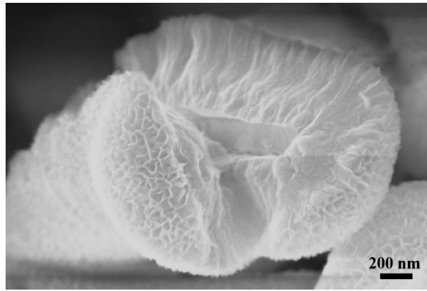
Fig. S4 Top view SEM image of the broken ZnIn 2 S 4 sample in 2 h reaction.
